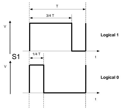
Figure 8.1: Bit-coding of S1
