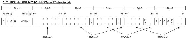
Figure 11.2: Example for a Type A aligned CLT frame
