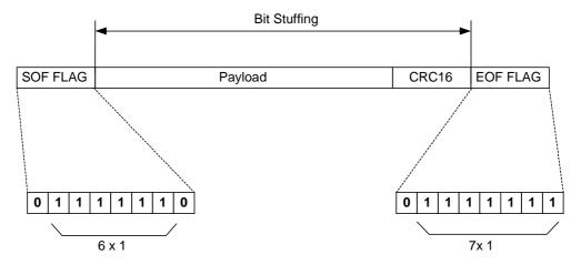
Figure 9.2: Frame structure sent by master
