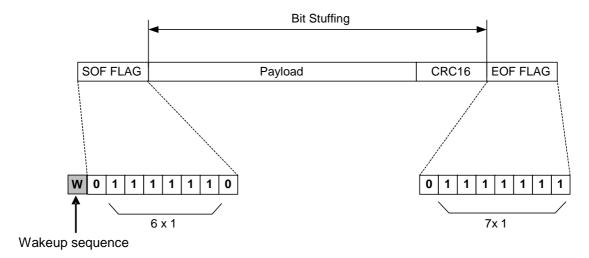
Figure 9.3: Frame structure sent by slave
