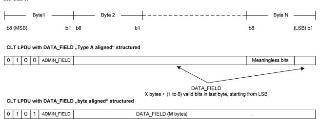
Figure 11.1: Typical examples for CLT frames with DATA\_FIELD present
