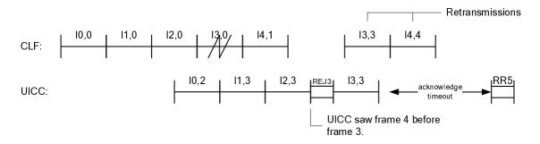
Figure 10.14: Piggybacking with reject frame after mismatching sequence number
