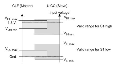
Figure 7.1: Voltage definitions for the signal S1
