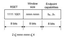
Figure 10.2: RSET frame payload
