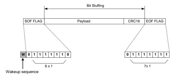
Figure 9.3: Frame structure sent by slave
