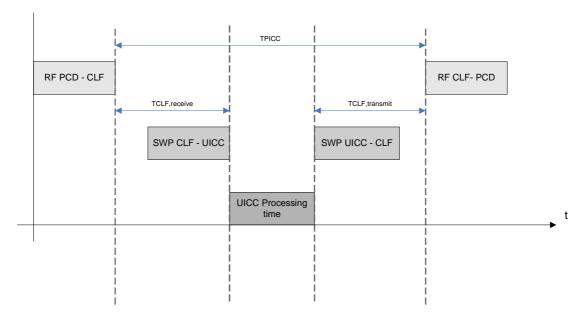
NOTE: SWP CLF-UICC and SWP UICC-CLF represent the time taken to transmit the data over SWP and are included in the T<sub>CLF,receive</sub> and T<sub>CLF,transmit</sub> times.
