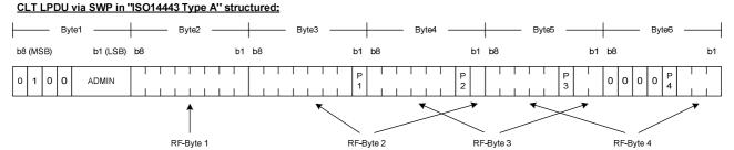
Figure 11.2: Example for a Type A aligned CLT frame
