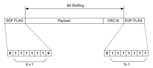
Figure 9.2: Frame structure sent by master
