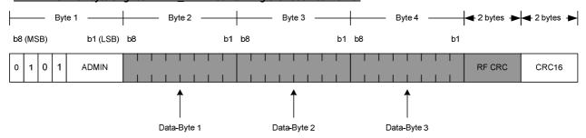
Figure 11.4: ISO/IEC 18092 [8] 212 kbps/424 kbps passive mode byte arrangement in a CLT frame (example)
