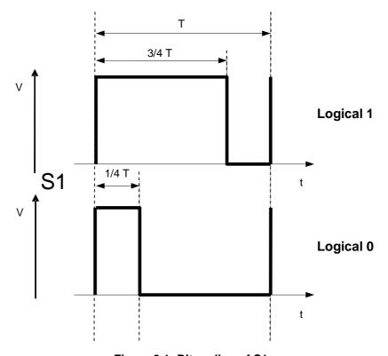
Figure 8.1: Bit-coding of S1
