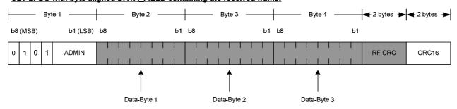
Figure 11.4: ISO/IEC 18092 [8] 212/424 kbps passive mode byte arrangement in a CLT frame (example)
