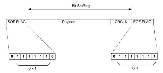
Figure 9.2: Frame structure sent by master
