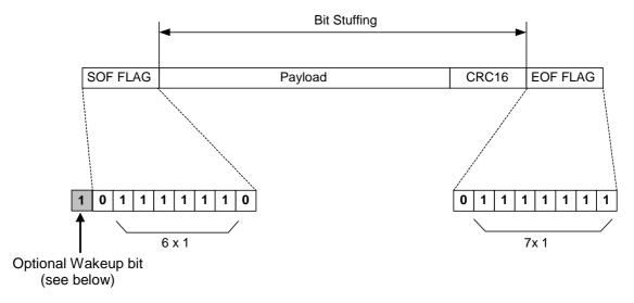
Figure 9.3: Frame structure sent by slave
