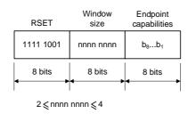
Figure 10.2: RSET frame payload
