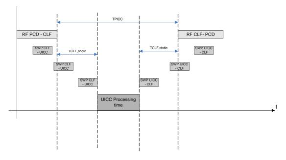
Figure 12.5: SHDLC transmission timings
