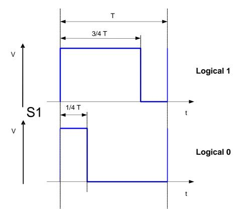
Figure 8.1: Bit-coding of S1
