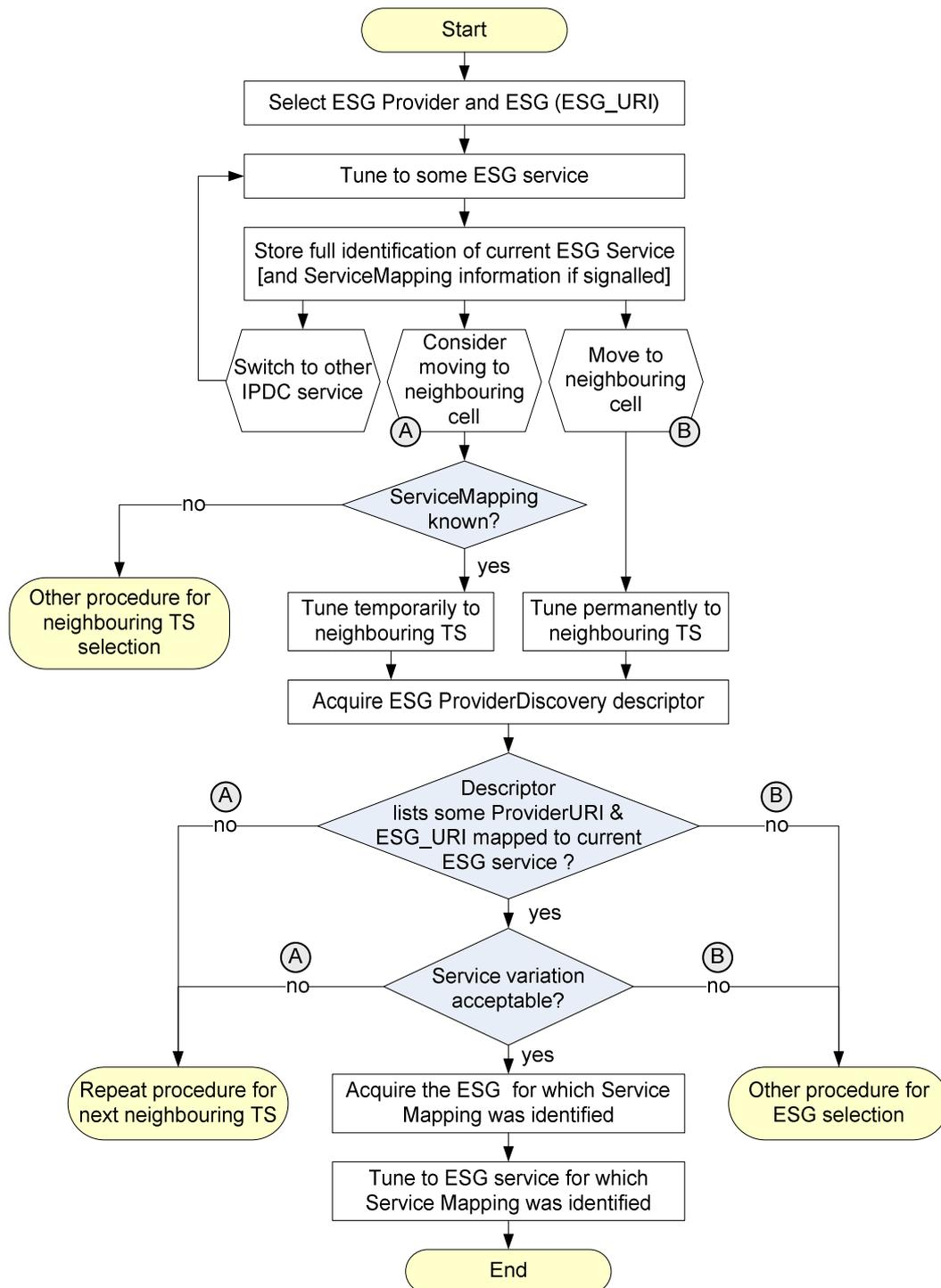
**Figure 28: Terminal procedure for ServiceMapping handling**
