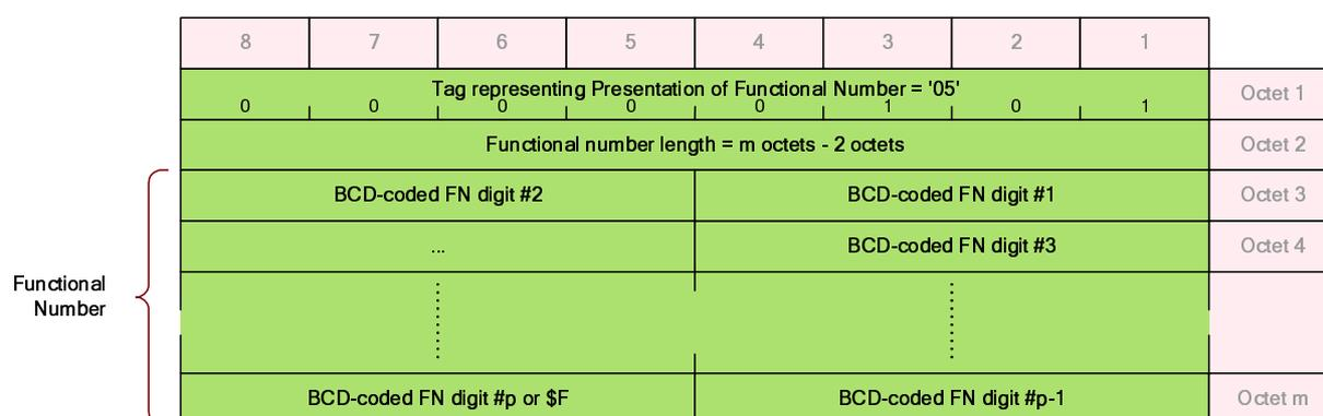
NOTE 1: The FN length field specifies the number of octets present to carry the FN. Each digit of a FN is encoded as a BCD digit (one nibble). The first FN digit is in bits 1 to 4 and the next digit is in bits 5 to 8 of octet 3 of the tag; the following digit is in bits 1 to 4 of next octet and so on. If the FN consists of an odd number of digits, then the last half octet (bits 4 to 7) of the FN should contain "\$F" as a filler. Therefore "\$F" can never be a valid digit within the FN.
