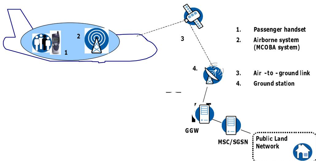
**Figure A.1-1: Overview of the MCOBA system and associated terrestrial components**
