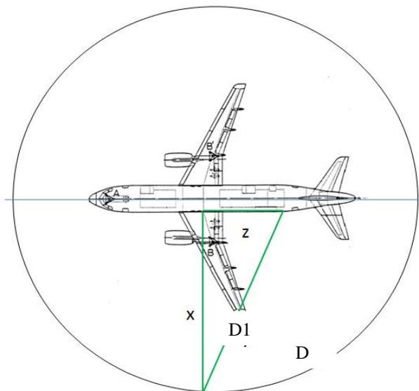
**Figure 5.4.3-1: Calculation of separation distance**
