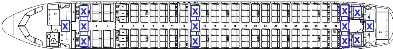
**Figure 5.1-1: Example of principle aircraft layout for narrow body aircraft type in standard cabin configuration with example measurement locations**
