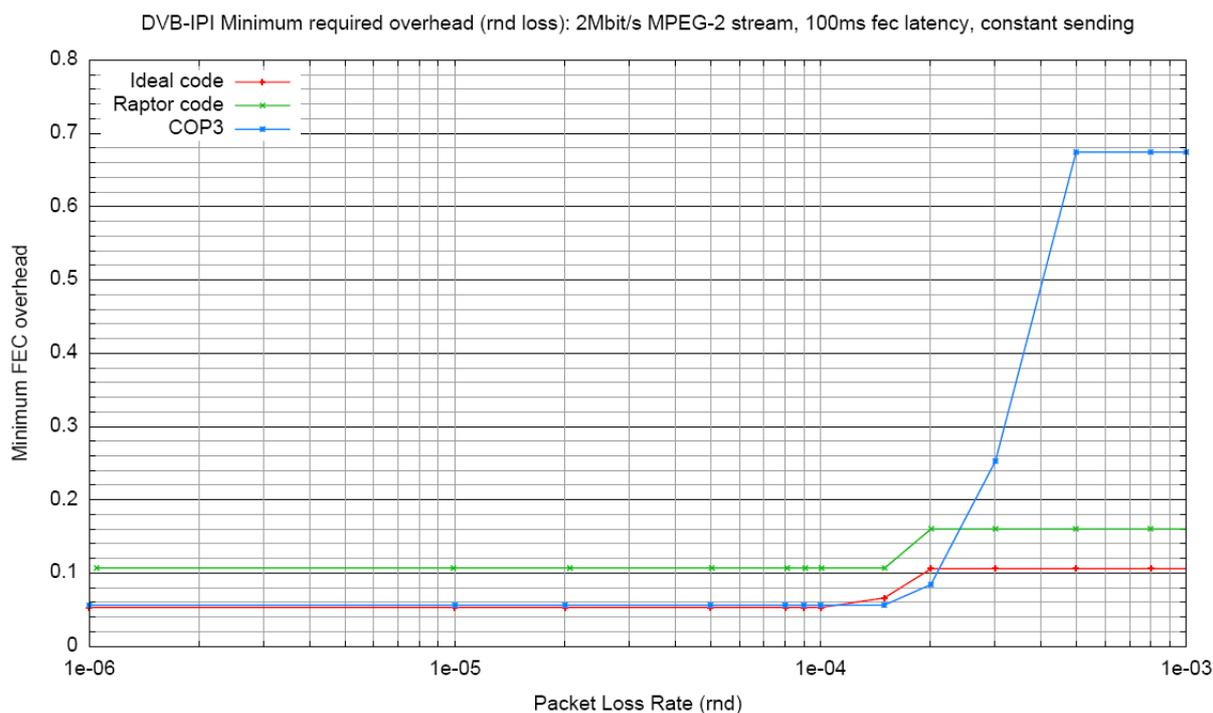
**Figure A.6.3.3.2.1-1: 2 Mbit/s MPEG-2 Transport Stream, 100 ms latency (live content), random loss, constant sending**
