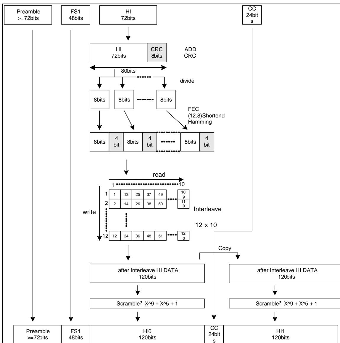
NOTE: Header Frame Channel Coding.
