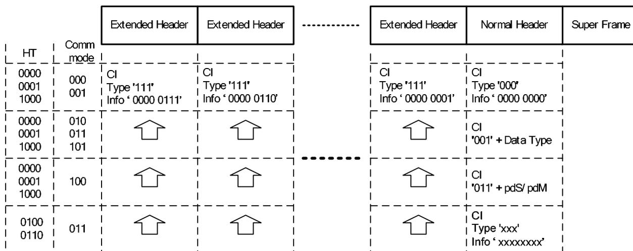
**Figure 12: Extended header coding**
