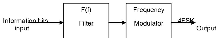
**Figure 13: 4FSK Modulator**
