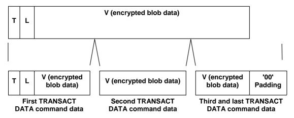
Figure 10.1: An example showing the splitting of an encrypted blob TLV into three TRANSACT DATA commands.
