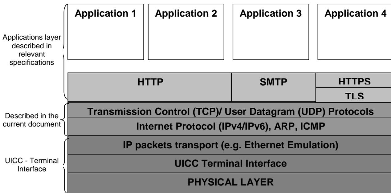
Figure 5: TCP/IP over UICC-Terminal Interface protocol stack
