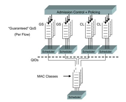
Figure 7.3: Intserv with SD "aggregated flow" classes
