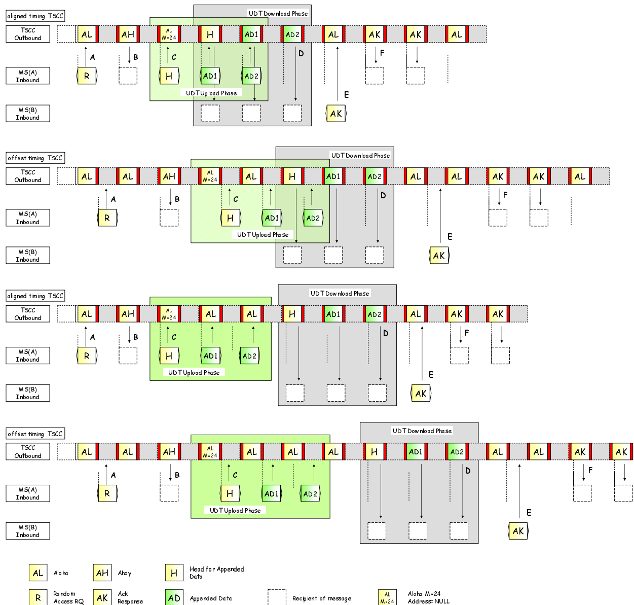
Figure 6.50: More Examples of a UDT Short Data Message transfer
