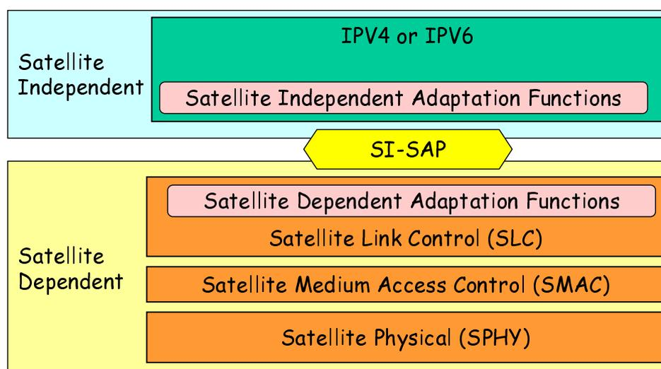
**Figure 2: Satellite Independent Service Access Point (SI-SAP)
