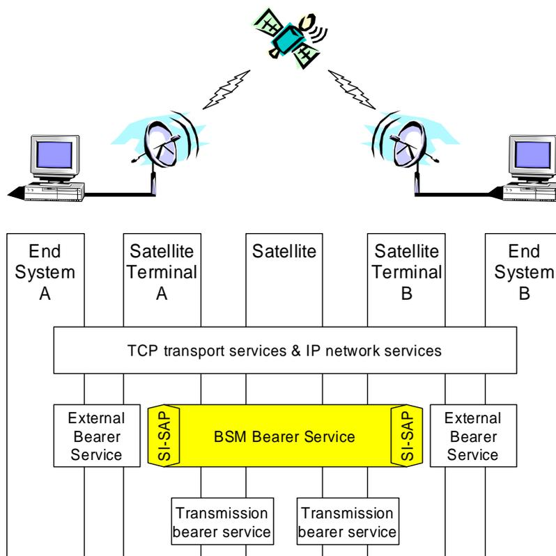
**Figure 1: Satellite Independent Service Access Point (SI-SAP)**
