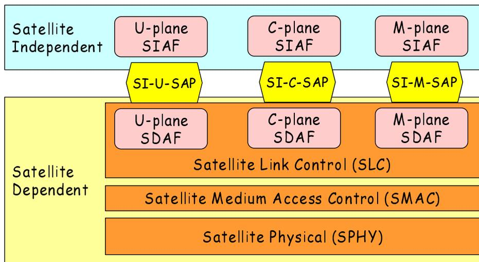
**Figure 3: Satellite Independent Service Access Point (SI-SAP)
