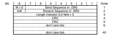
Figure 13: Synchronization frame format type DFFU10
