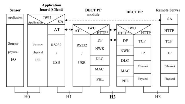
NOTE: This scenario assumes that FP has sufficient knowledge about the addressing needed to communicate with the remote client.
