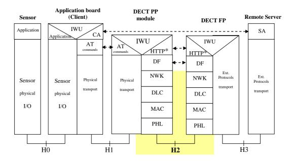
Figure 1: Basic system architecture reference configuration
