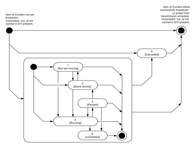
Figure 18: TVA\_id UML state diagram
