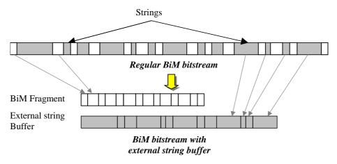
Figure 12: BiM bitstream with an external string buffer
