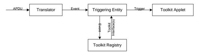
Figure 3: Toolkit applet triggering diagram
