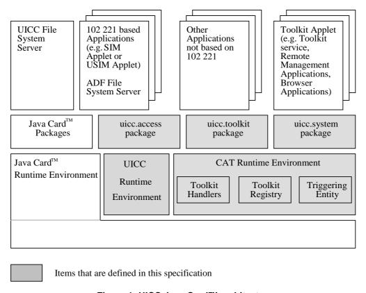
Figure 1: UICC Java Card™ architecture
