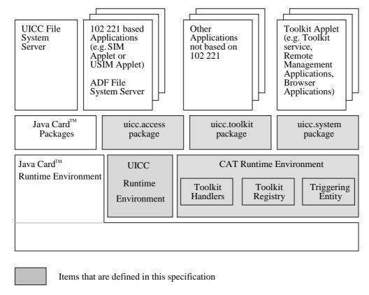
Figure 1: UICC Java Card™ architecture
