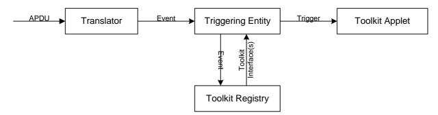
Figure 3: Toolkit applet triggering diagram
