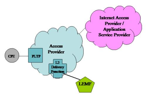
Figure 2: Scenario in which access is offered by a provider separate from the one that is offering Internet transport and application service
