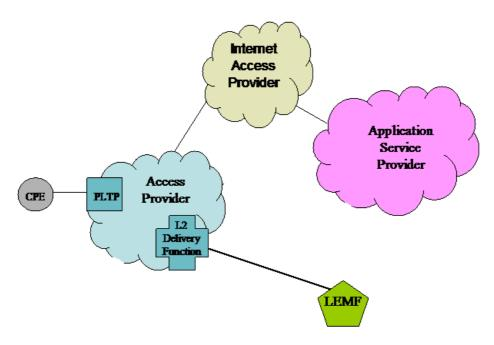
Figure 1: Scenario in which access, transport and application services are offered by three different providers
