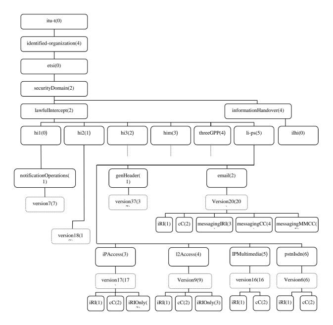
Figure A.1: Object identifier tree
