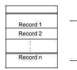
Figure 8.3: Structure of a cyclic file
