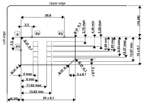
Figure 4.1: Plug-in UICC
