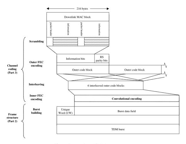
Figure 5.3.3.1: Downlink data structures
