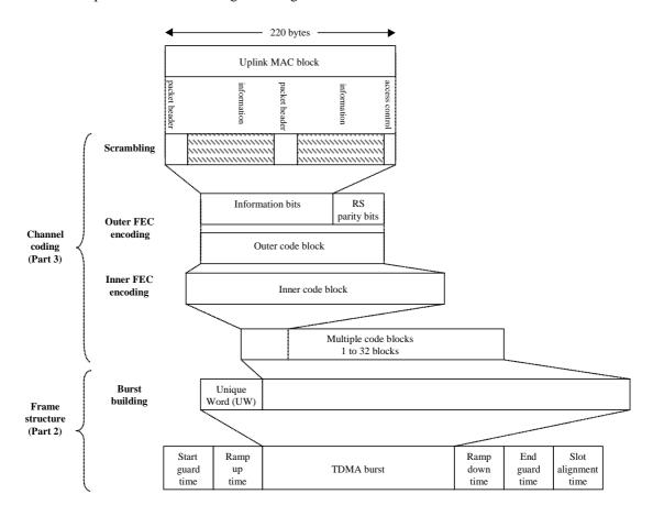
Figure 5.3.2.1: Uplink data structures
