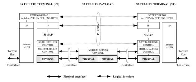
Figure 4.3: Air interface architecture
