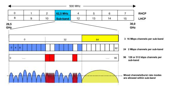
Figure 5.3.2.7: Possible arrangement of uplink carriers within a sub-band
