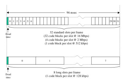
Figure 5.3.2.4: Uplink frame structure
