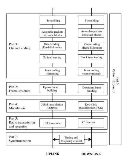
Figure 5.3.1: Physical layer functions
