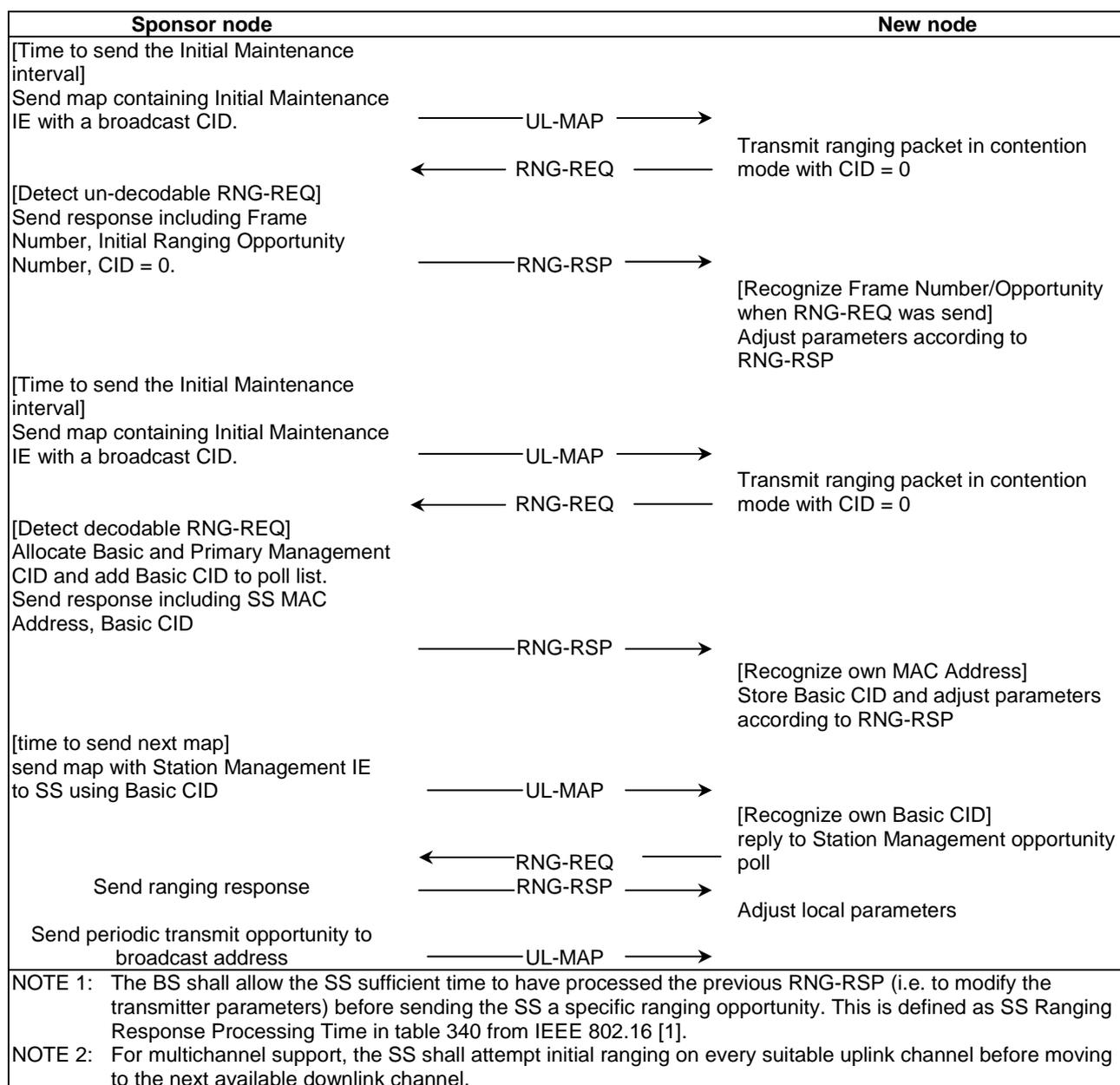
On receiving a RNG-RSP instruction to move to a new downlink frequency and/or uplink channel ID, the SS shall consider any previously assigned Basic, Primary Management, and Secondary Management CIDs to be de assigned, and shall obtain new Basic, Primary Management, and Secondary Management CIDs via initial ranging and registration.
