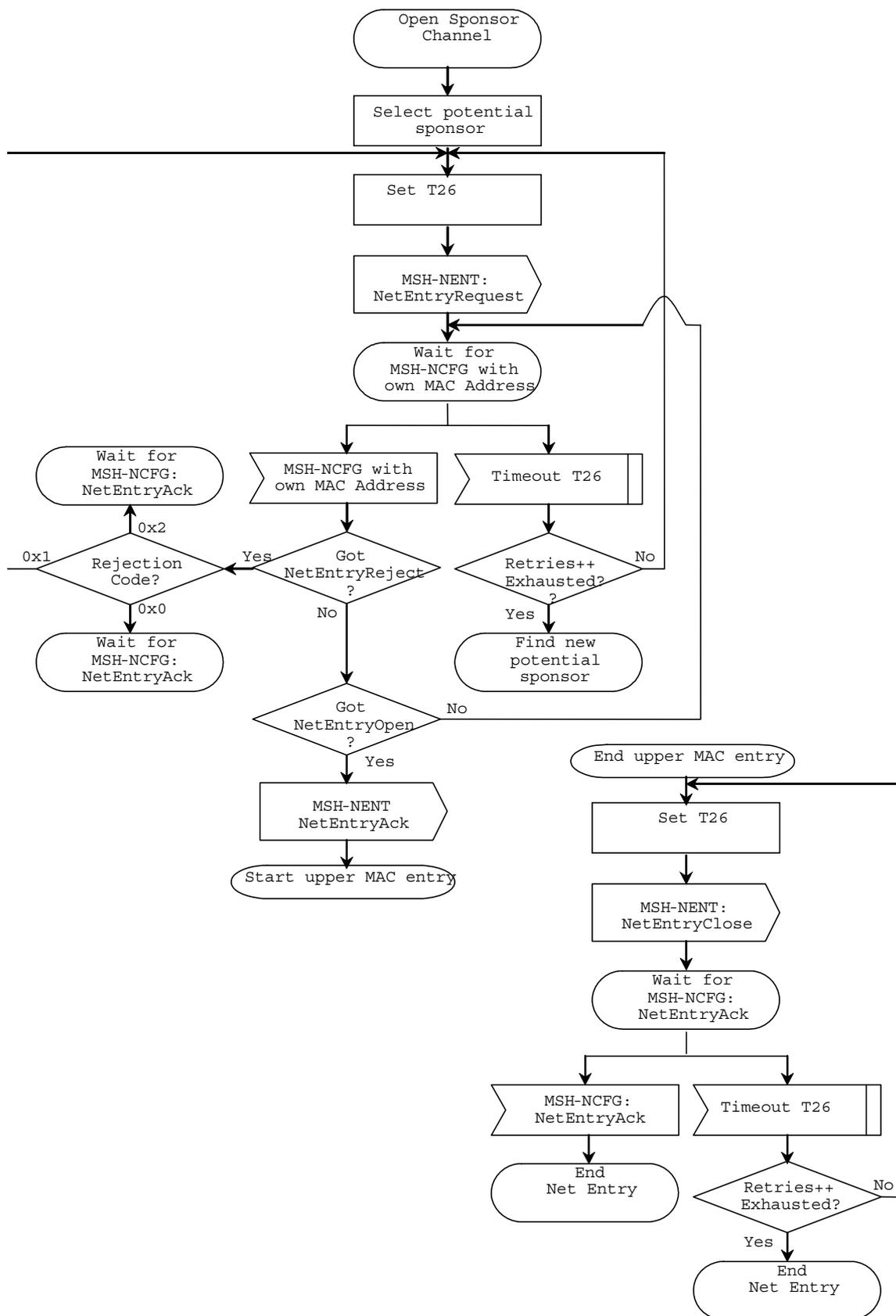
Figure 11: Synchronization and network entry - new node II
