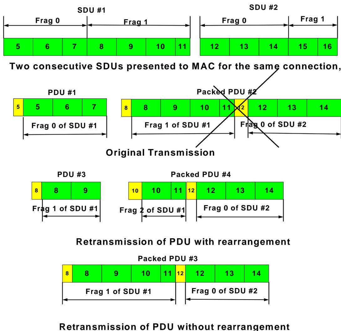
Figure 4: Block usage examples for ARQ transmissions and retransmissions
