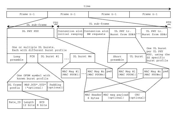
Figure 12: Example of OFDM PMP frame structure with TDD
