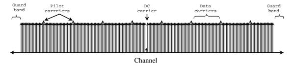
Figure 2: OFDM symbol frequency structure
