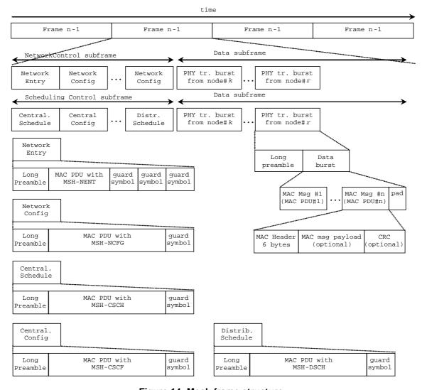
Figure 14: Mesh frame structure
