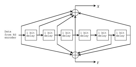
Figure 6: Convolutional encoder of rate 1/2
