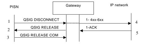
Figure 10: Typical message sequence for call clearing from QSIG to SIP, during establishment of a call from SIP to QSIG (gateway has not sent a final response to the SIP INVITE request)
