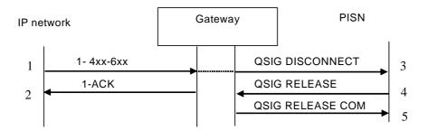
Figure 13: Typical message sequence for call clearing from SIP to QSIG, during establishment of a call from QSIG to SIP (gateway has not previously received a final response to the SIP INVITE request)
