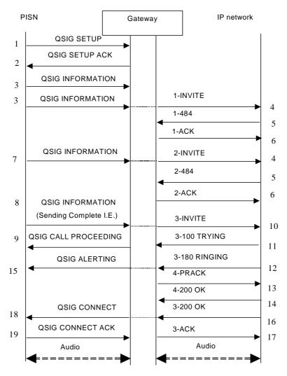
Figure 5: Typical message sequence for successful call establishment from QSIG to SIP, using overlap procedures on both QSIG and SIP
