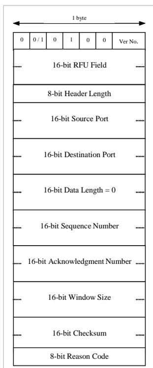
**Figure 43: RST PDU structure**
