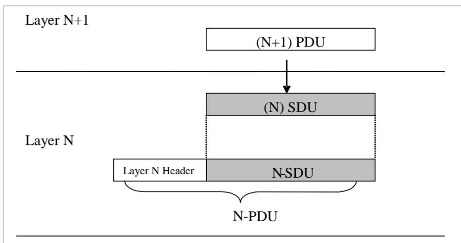
Figure 6: N-SDU and N-PDU with no segmentation
