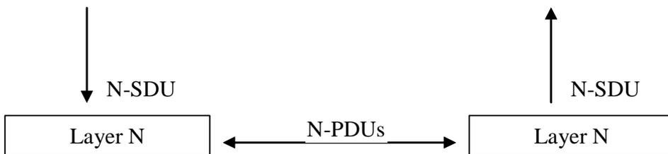
Figure 4: PDUs exchange between two Layers N
