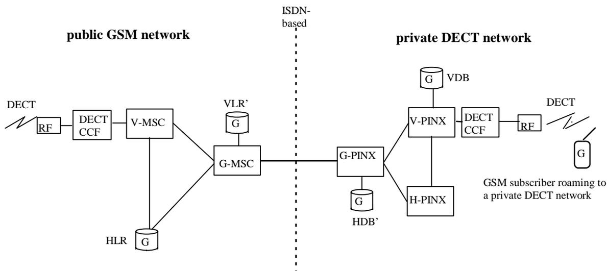
**Figure 2a: End-to-end Interworking Reference Configuration - Scenario 2a**
