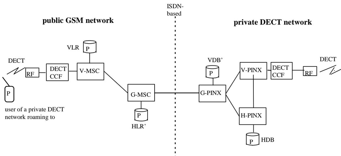
**Figure 2b: End-to-end Interworking Reference Configuration - Scenario 2b**
