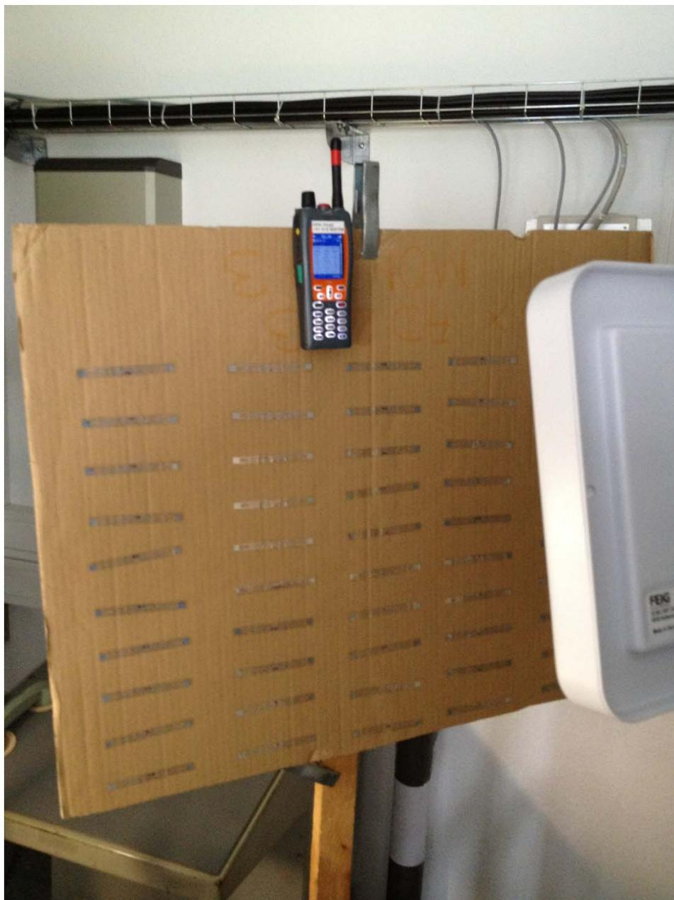
**Figure B.10: GSM-R mobile placed opposite of the demonstrator and just above the RFID tags**
