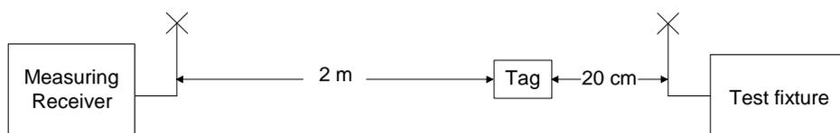
**Figure 4: Measurement of tag emissions**
