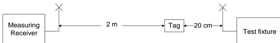
**Figure A.9: Measurement of Tag emissions**
