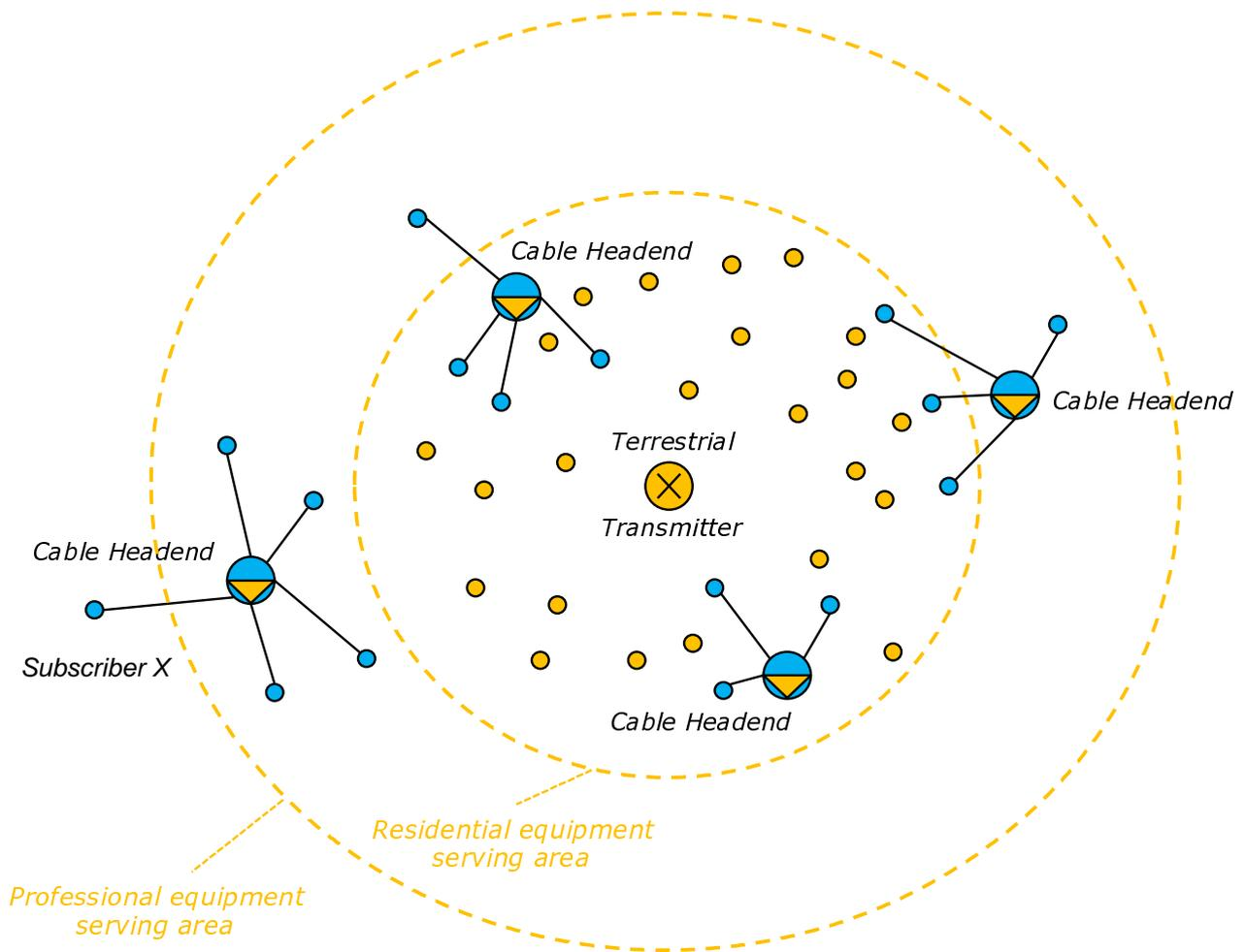
**Figure 3: Cable headends in- and outside the residential equipment serving area of a terrestrial TV transmitter**
