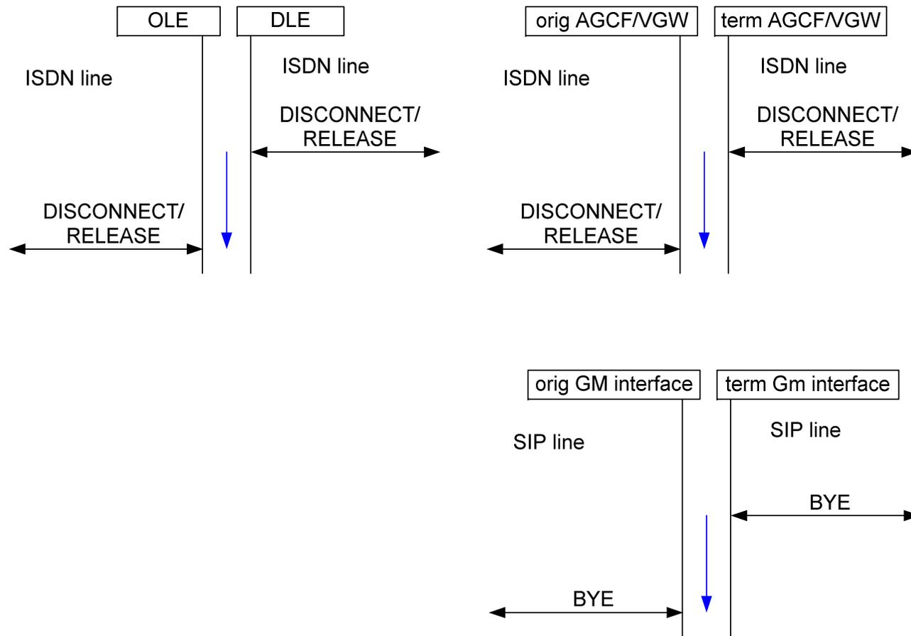
Figure 11: Connection call release delay
