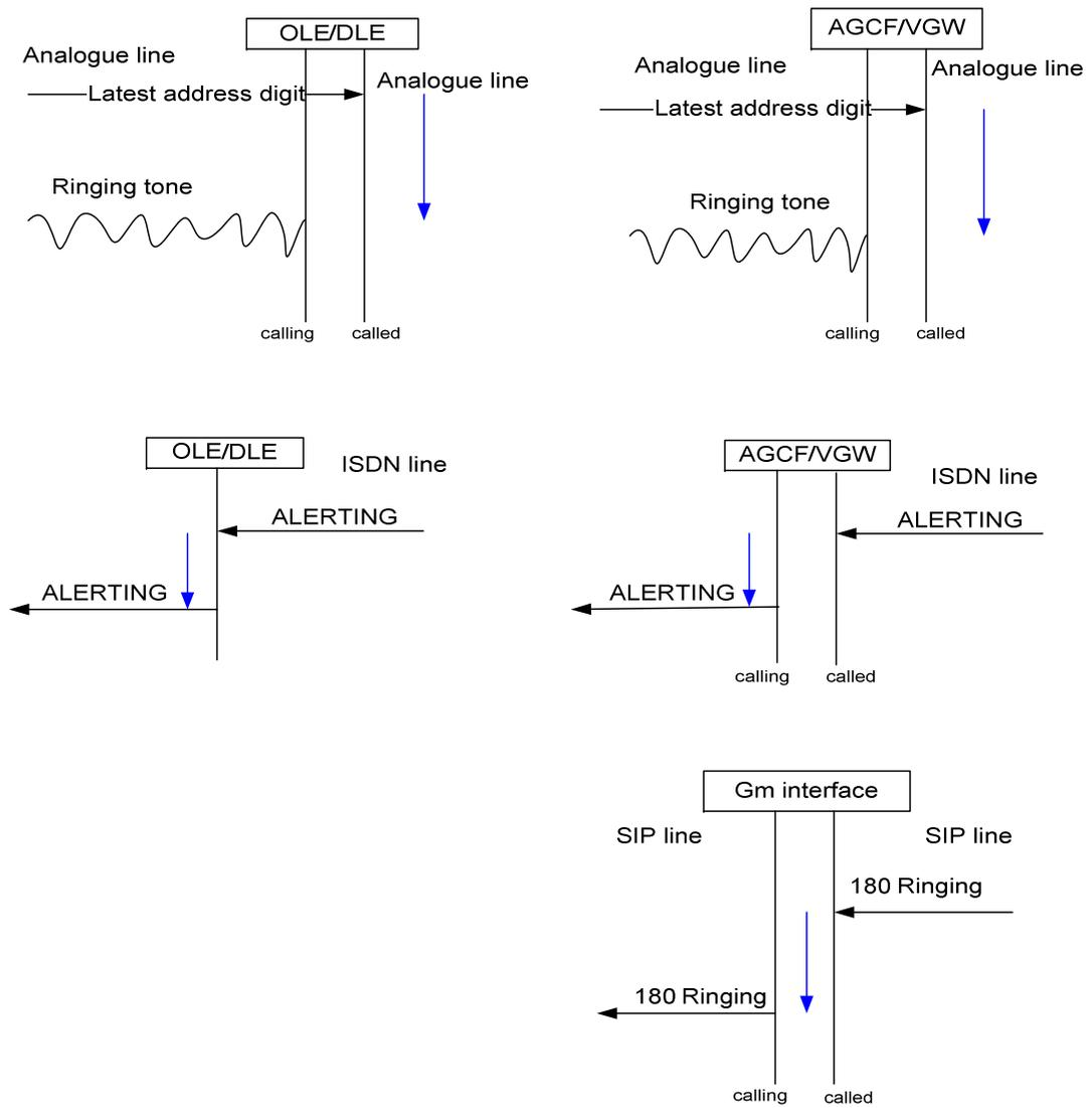
**Figure 7: Alerting sending delay for internal traffic
