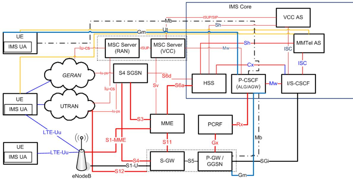
Figure 1: IMS/LTE Basic Configuration
