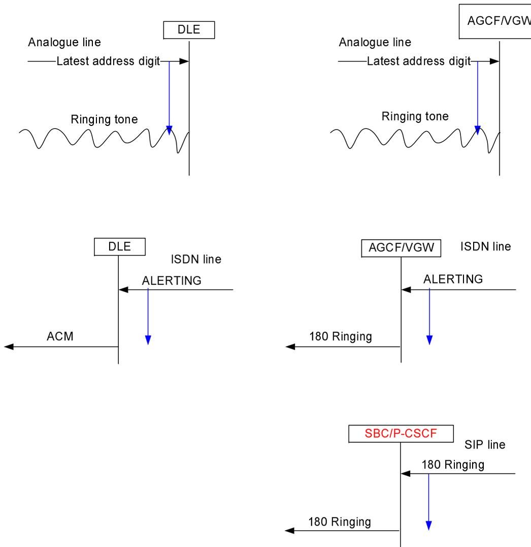
Figure 6: Local exchange Alerting sending delay for terminating traffic (in different locations)
