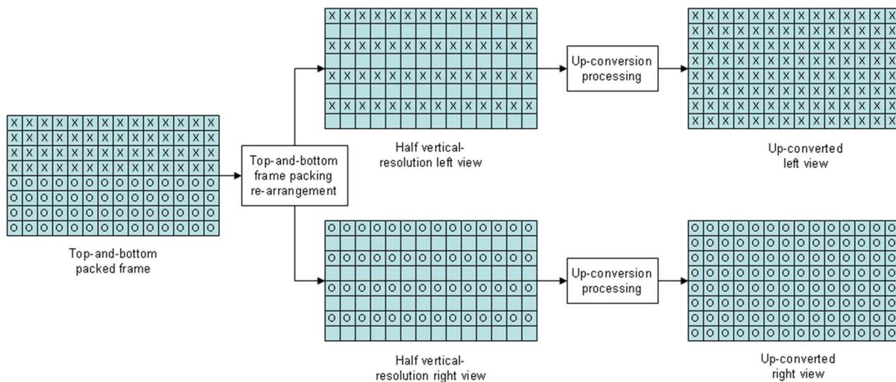
**Figure A.2: Top-and-Bottom decoded video frame decomposition**
