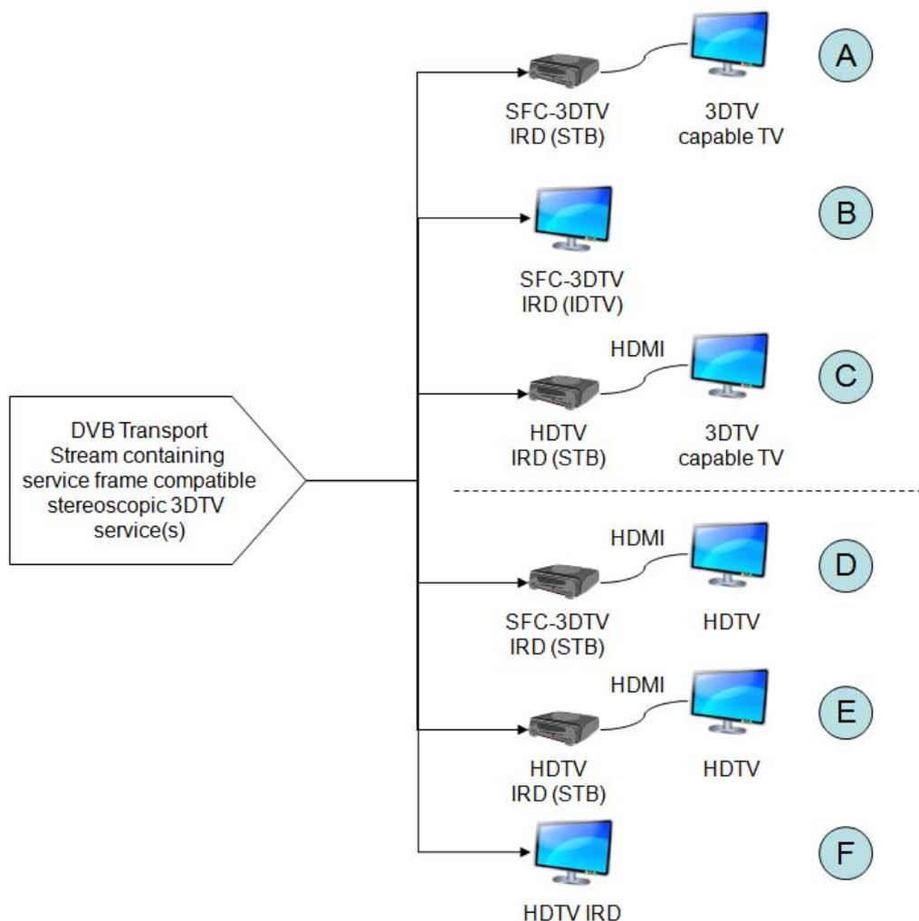
**Figure 3: Service frame compatible plano-stereoscopic 3DTV IRD scenarios**
