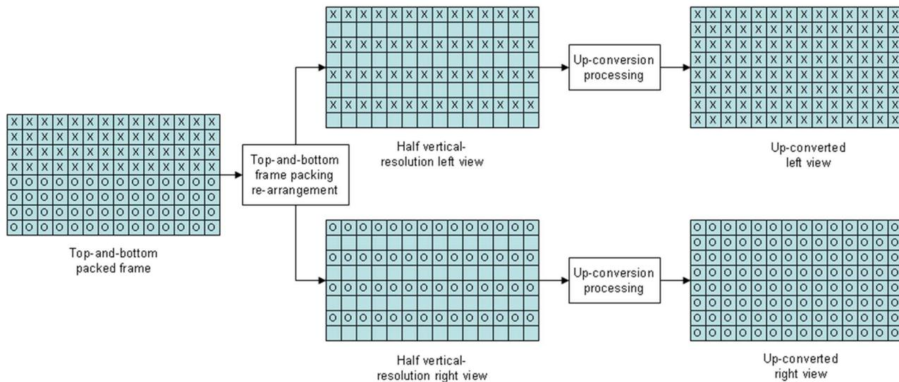
**Figure A.2: Top-and-Bottom decoded video frame decomposition**
