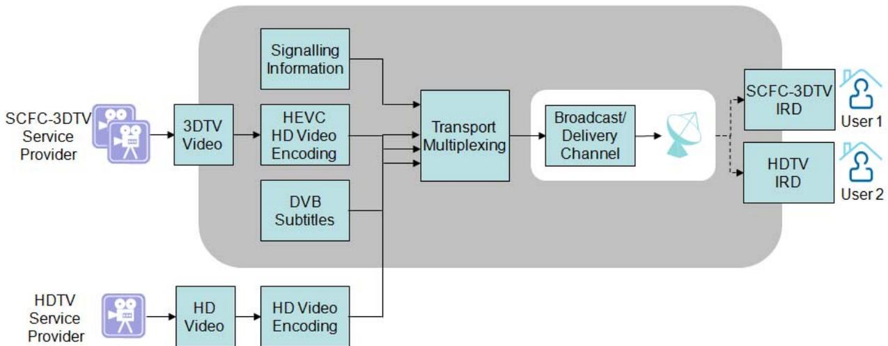
**Figure 1: Scope of the service frame compatible plano-stereoscopic 3DTV specification**
