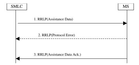
Figure 2.2: Assistance Data Delivery procedure
