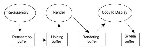
Figure 5.1: Simple profile Buffer management model for a MOT SlideShow decoder
