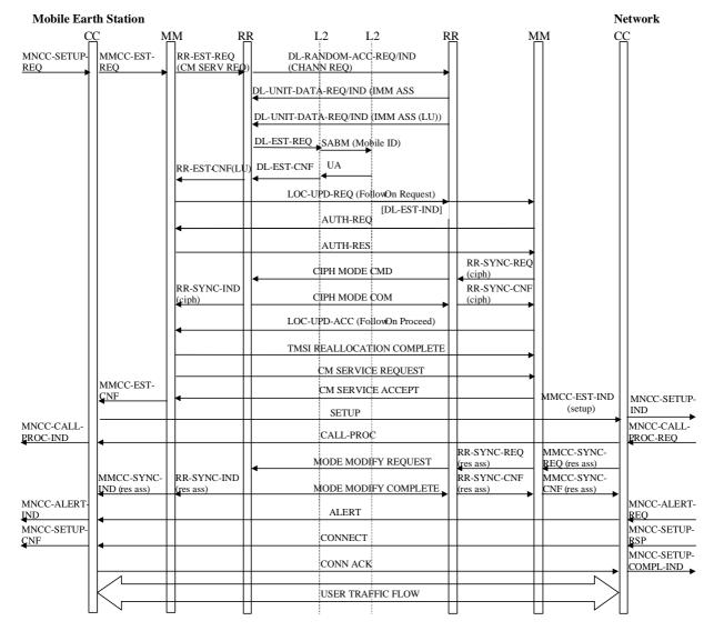
Figure A.8: Mobile-originated call setup with optimal routing. Successful case (see GMR-1 03.297[3])
