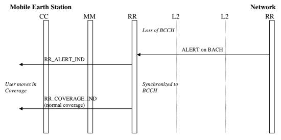
Figure A.9: Alerting. Successful case (see GMR-1 03.298 [4])
