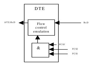
Figure 14: XON/XOFF Flow Control on input
