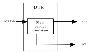
Figure 13: XON/XOFF Flow Control on input
