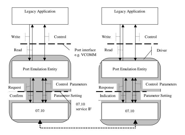
The legacy application utilises a conventional serial port communication interface. The port emulation entity maps a system specific communication interface to 07.10 services. The 07.10 provides several transparent data stream channels and a control channel. The port interface is the application programmers interface for communication. It varies from system to system and one example is Virtual comm ports in windows.
