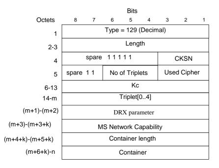
NOTE: k is the value of the MS Network Capability length indicator (GSM 04.08)
