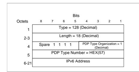
Figure 27: End User Address information element for IPv6
