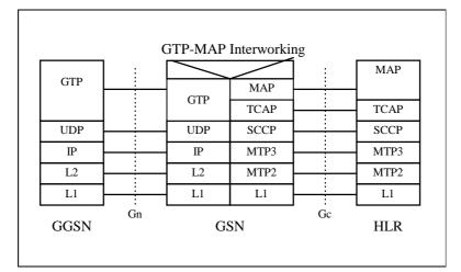
Figure 6: GGSN - HLR Signalling via a GTP-MAP protocol-converter in a GSN
