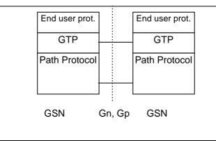
Figure 39: Transmission Plane - Protocol Stack
