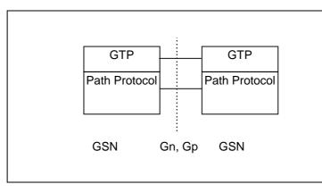
Figure 4: Signalling Plane - Protocol stack
