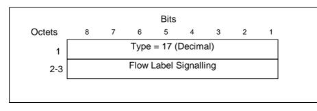
Figure 22: Flow Label Signalling information element
