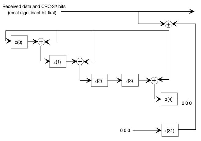
Figure A.1: 32-bit CRC decoder model
