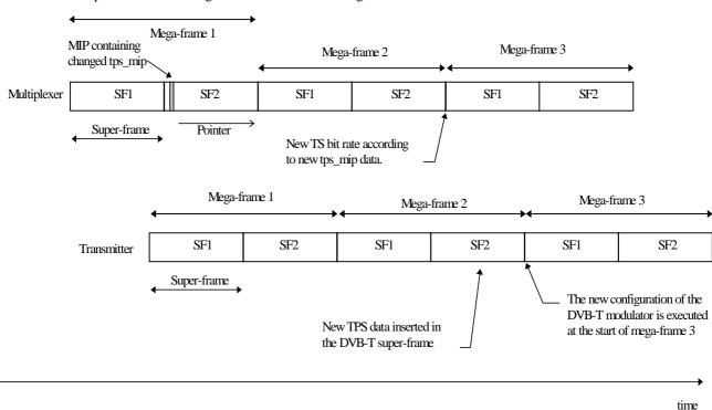
Figure C.1: Reconfiguration of DVB-T modulator parameters by using the MIP
