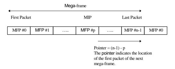
Figure 2: Overall mega-frame structure
