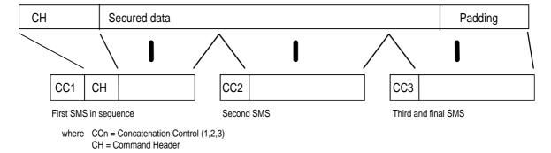
Figure 3: Example of command split using concatinated point to point SMS
