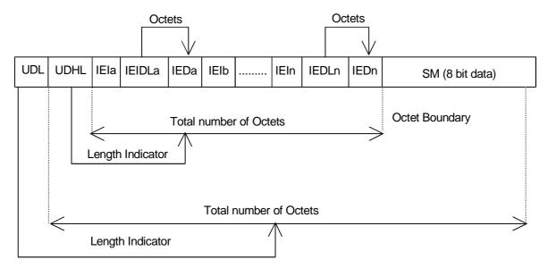
Figure 2: Structure of User Data Header in the Short Message Point to Point
