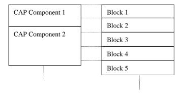
Figure 6: Relationship between CAP File components and Load File Blocks
