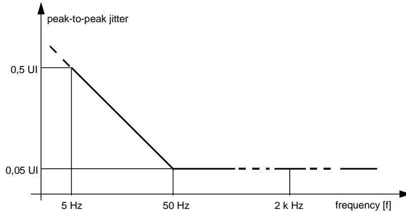
Figure 49E: Output jitter at ISDN-BA interface
