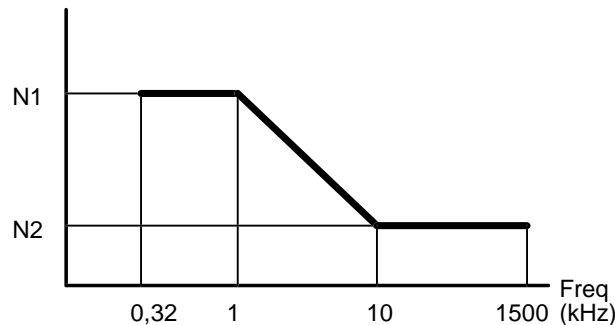
Figure 35: Test noise characteristics
