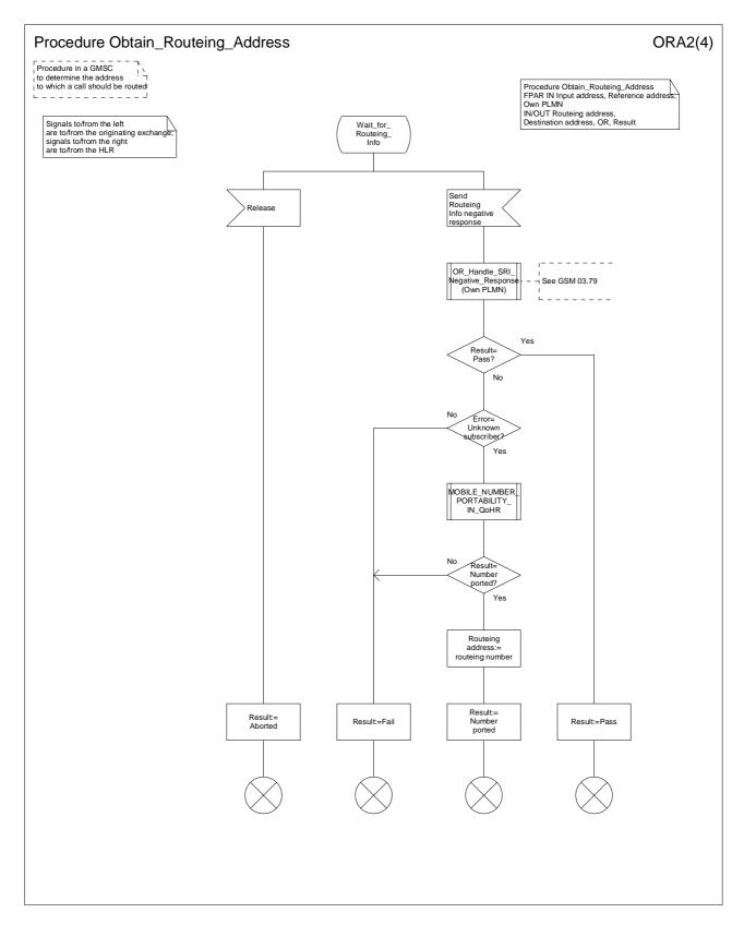
Figure 36b: Procedure Obtain\_Routeing\_Address (sheet 2)
