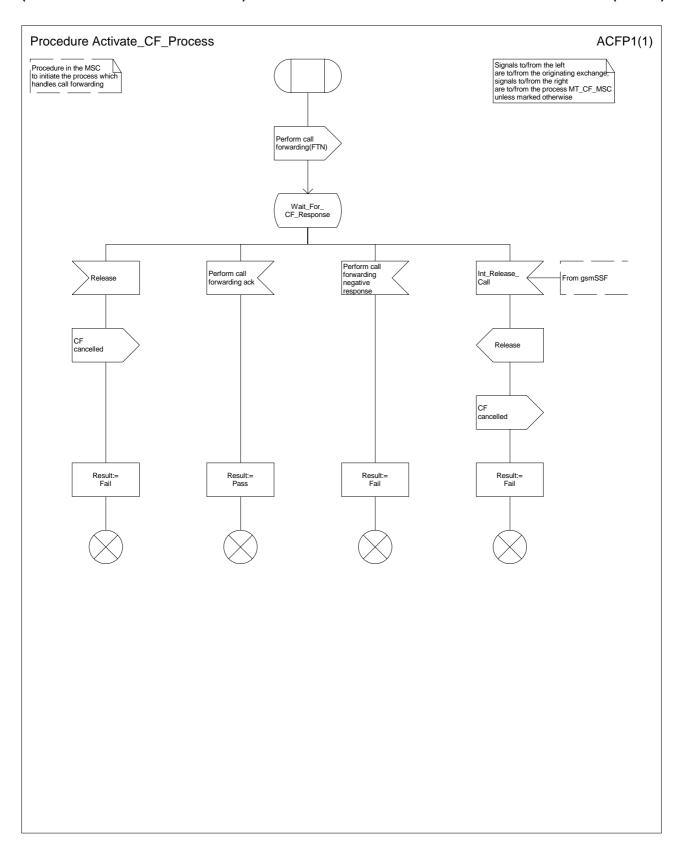
Figure 41: Procedure Activate\_Call\_Forwarding\_Process
