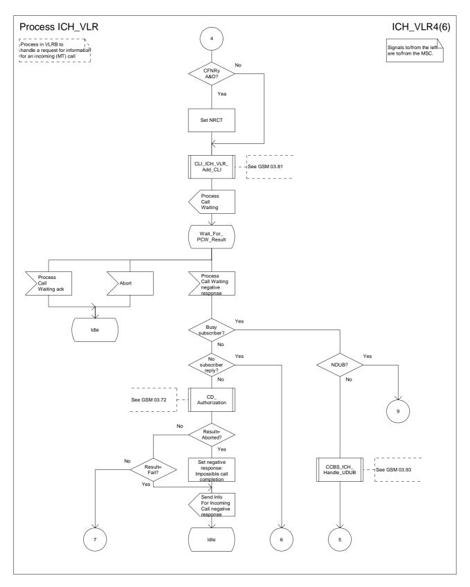
Figure 69d: Process ICH\_VLR (sheet 4)
