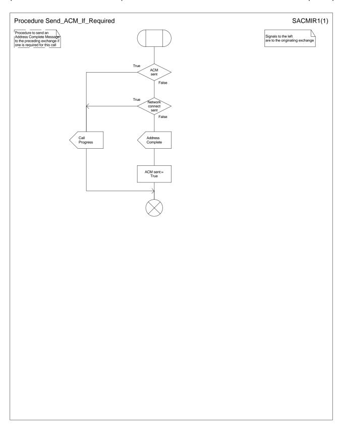
Figure 37: Procedure Send\_ACM\_If\_Required
