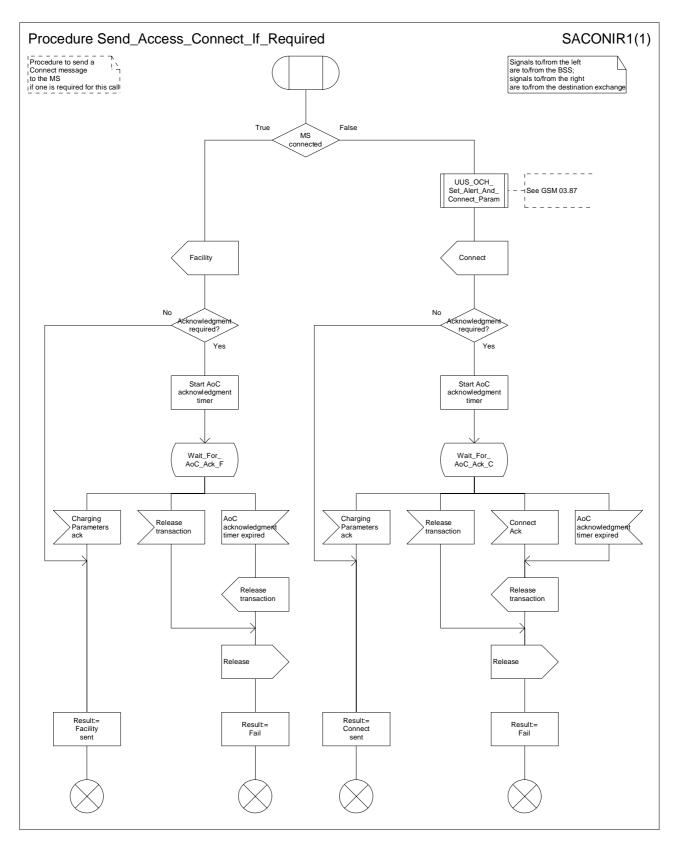
Figure 18: Procedure Send\_Access\_Connect\_If\_Required
