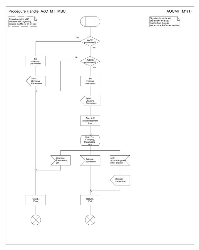
Figure 67: Procedure Handle\_AoC\_MT\_MSC
