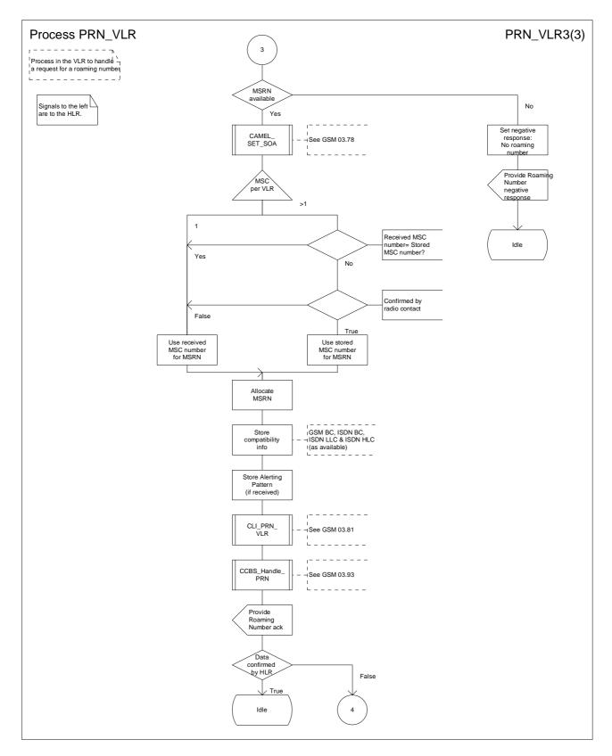
Figure 54c: Process PRN\_VLR (sheet 3)
