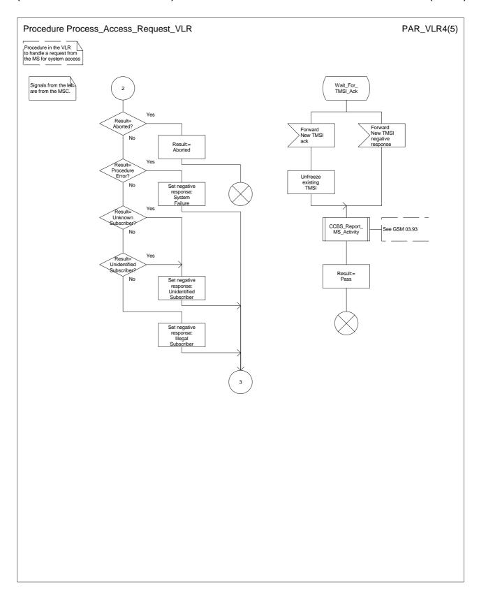
Figure 20d: Procedure Process\_Access\_Request\_VLR (sheet 4)
