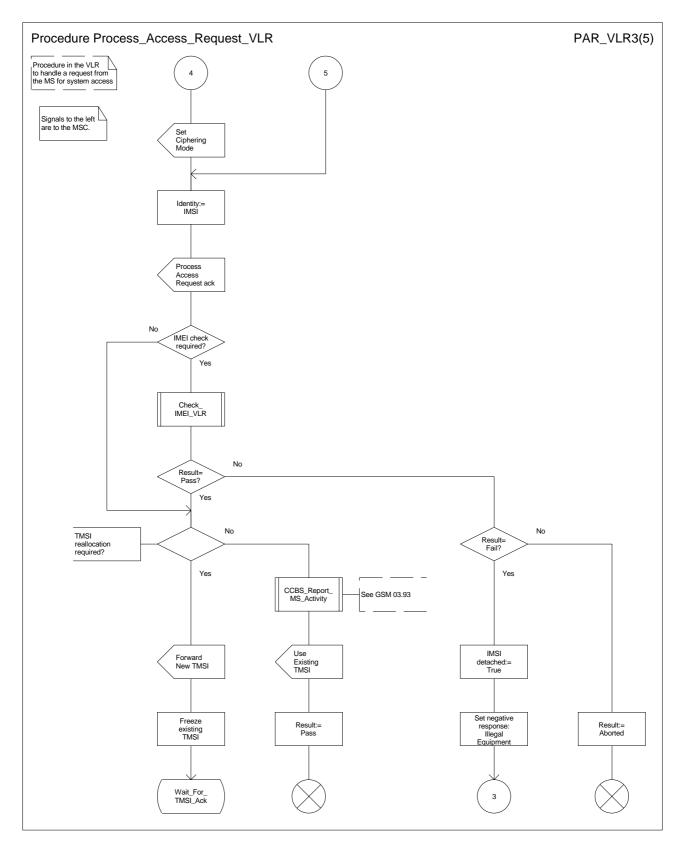
Figure 20c: Procedure Process\_Access\_Request\_VLR (sheet 3)
