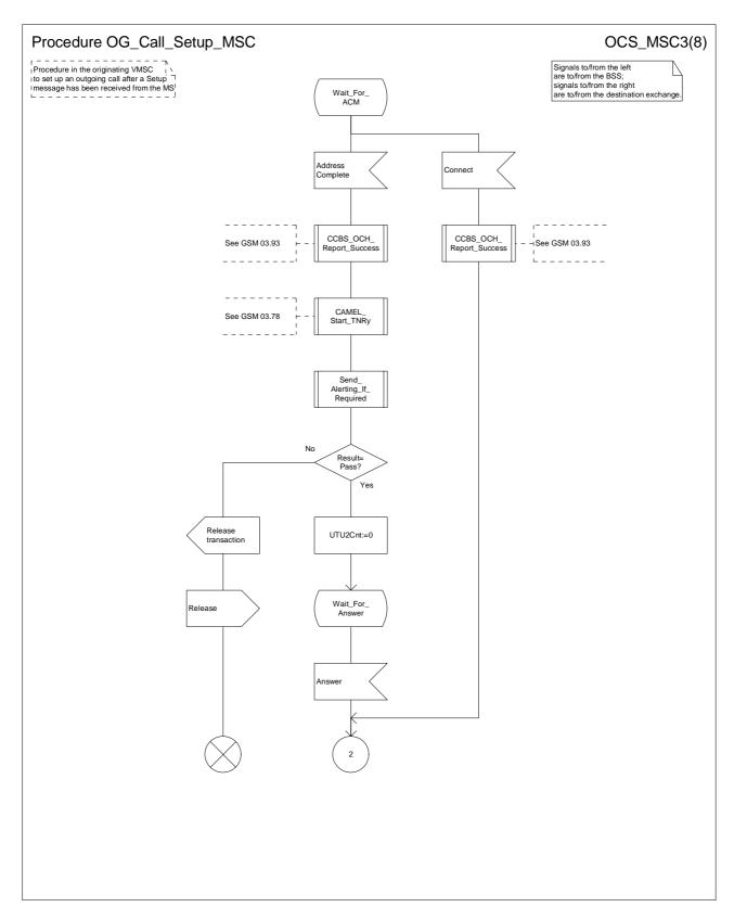
Figure 8c: Procedure Outgoing\_Call\_Setup \_MSC (sheet 3)
