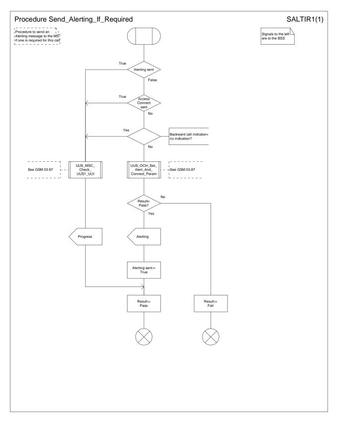
Figure 15: Procedure Send\_Alerting\_If\_Required
