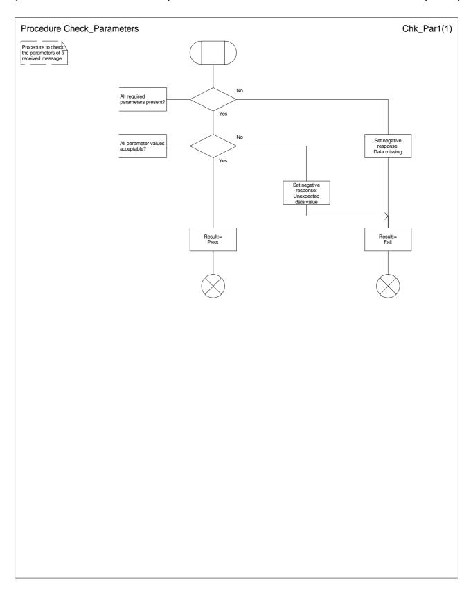
Figure 44: Procedure Check\_Parameters
