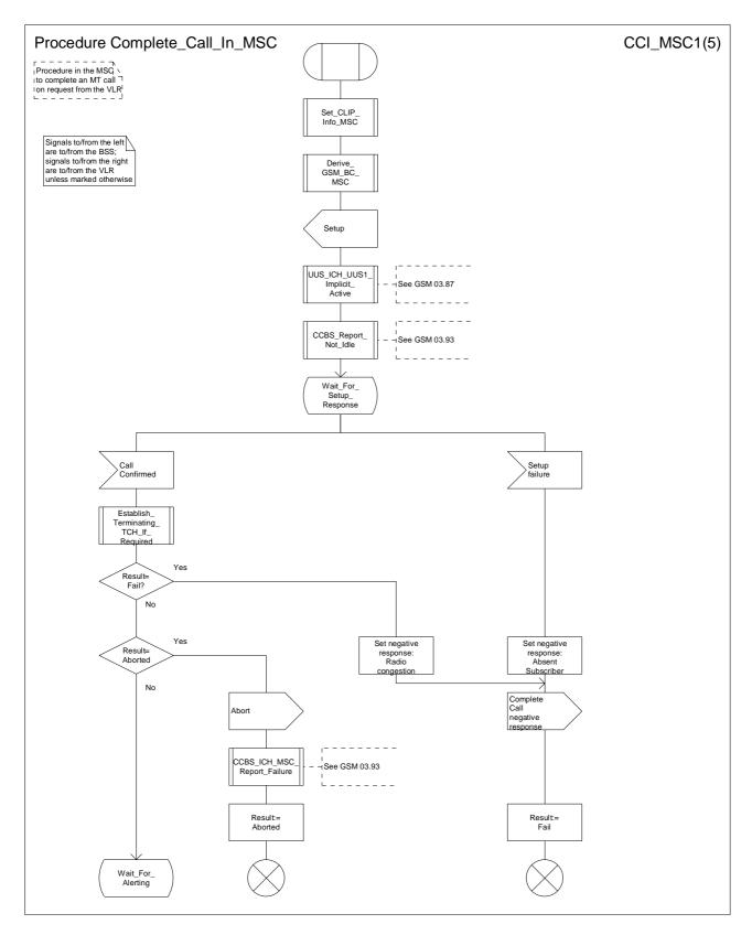
Figure 62a: Procedure Complete\_Call\_In\_MSC (sheet 1)
