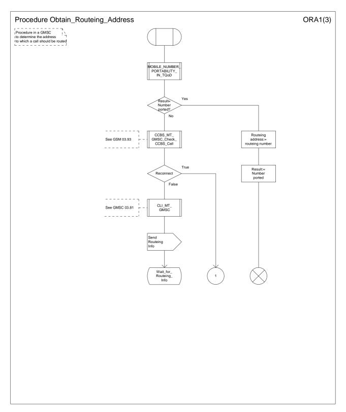
Figure 36a: Procedure Obtain\_Routeing\_Address (sheet 1)
