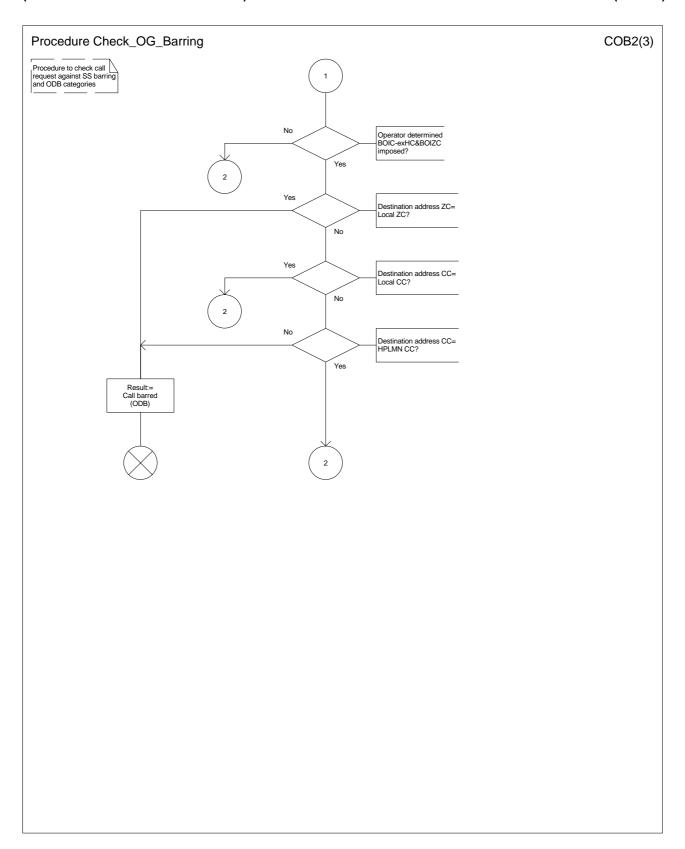
Figure 34b: Procedure Check\_OG\_Barring (sheet 2)
