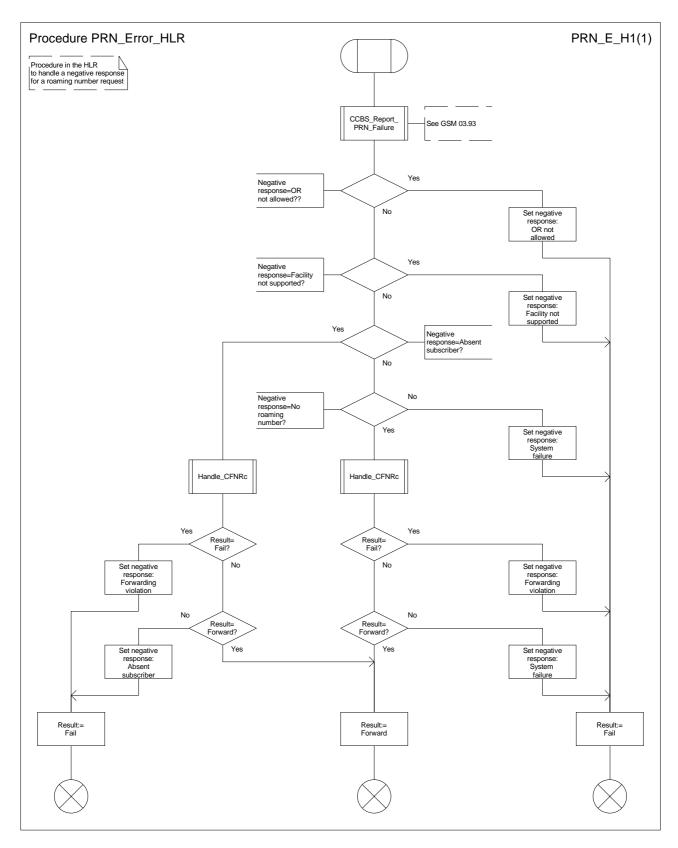
Figure 47: Procedure PRN\_Error\_HLR
