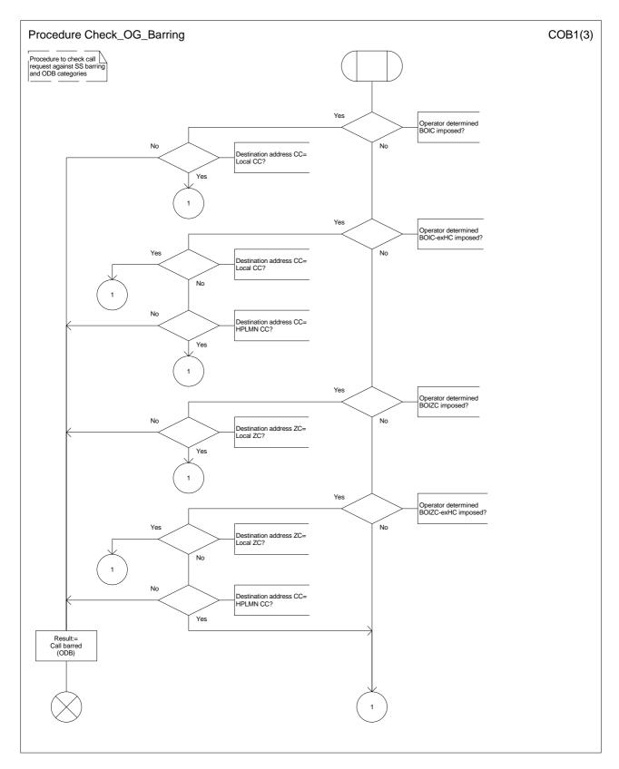
Figure 34a: Procedure Check\_OG\_Barring (sheet 1)
