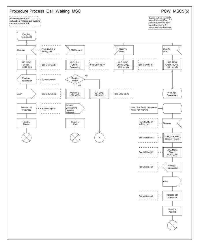
Figure 63e: Procedure Process\_Call\_Waiting\_MSC(sheet 5)
