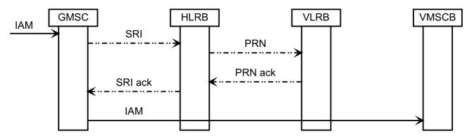
Figure 4: Information flow for retrieval of routeing information for a basic mobile terminated call
