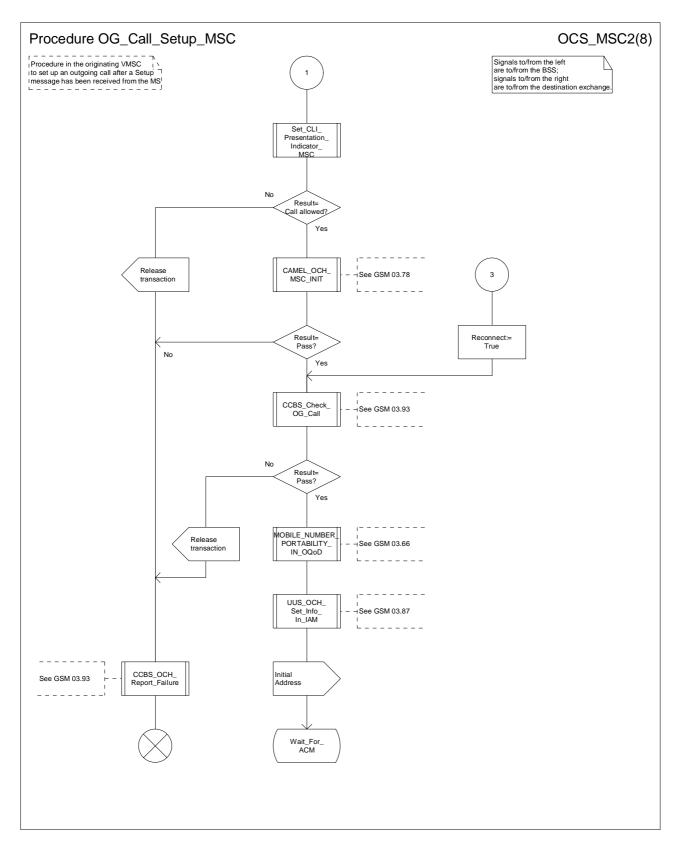
Figure 8b: Procedure Outgoing\_Call\_Setup \_MSC (sheet 2)
