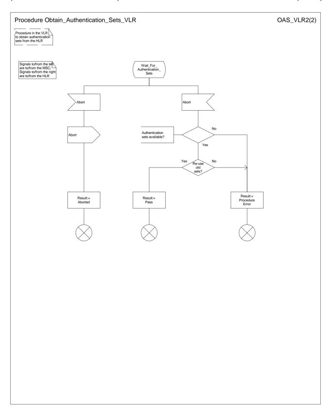
Figure 25b: Procedure Obtain\_Authentication\_Sets\_VLR (sheet 2)
