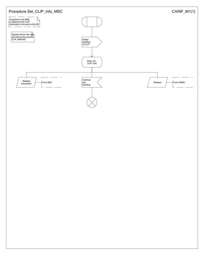
Figure 64: Procedure Set\_CLIP\_Info\_MSC
