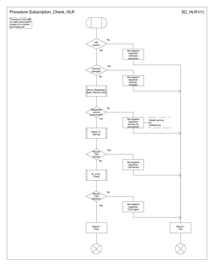
Figure 45: Procedure Subscription\_Check\_HLR
