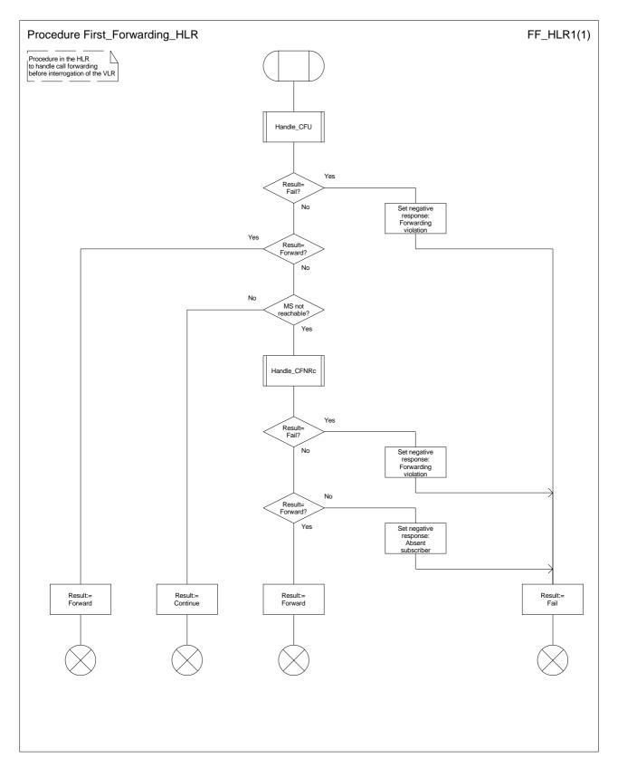
Figure 46: Procedure First\_Forwarding\_HLR
