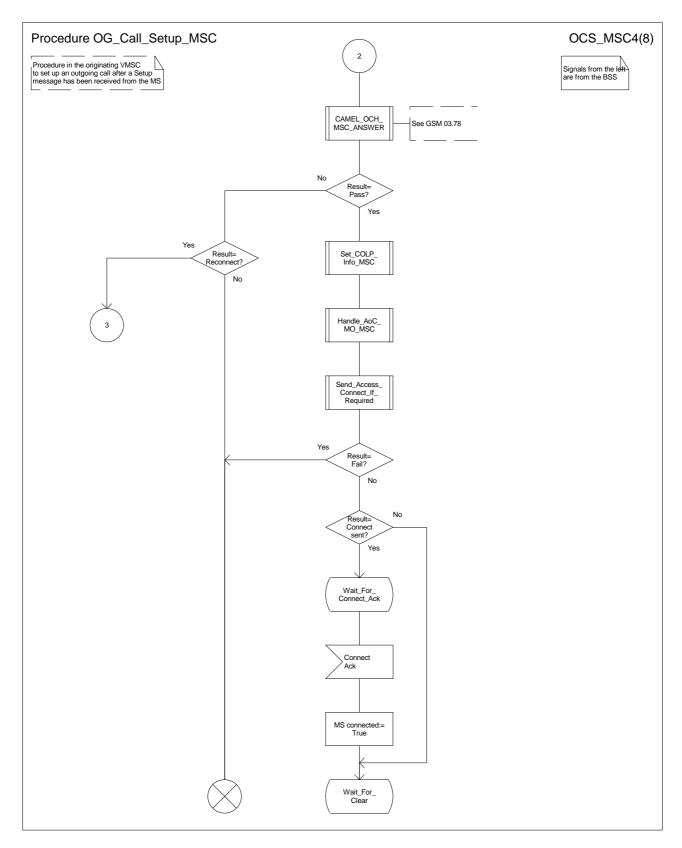
Figure 8d: Procedure Outgoing\_Call\_Setup \_MSC (sheet 4)
