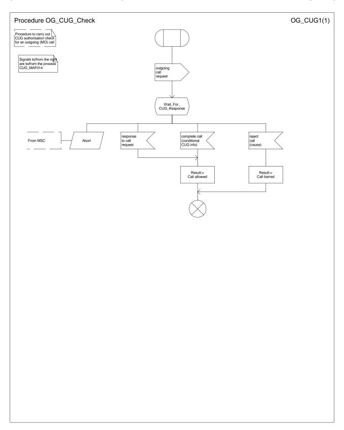
Figure 31: Procedure OG\_CUG\_Check
