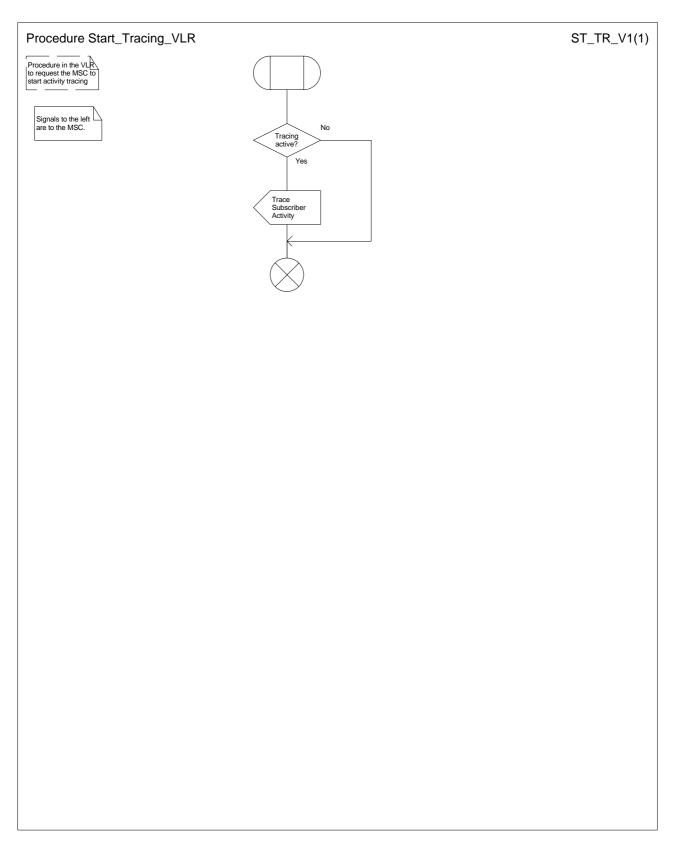
Figure 26: Procedure Start\_Tracing\_VLR
