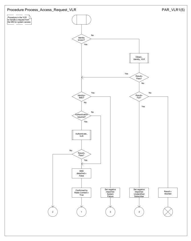
Figure 20a: Procedure Process\_Access\_Request\_VLR (sheet 1)
