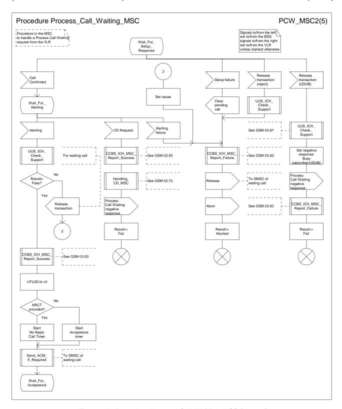
Figure 63b: Procedure Process\_Call\_Waiting\_MSC (sheet 2)
