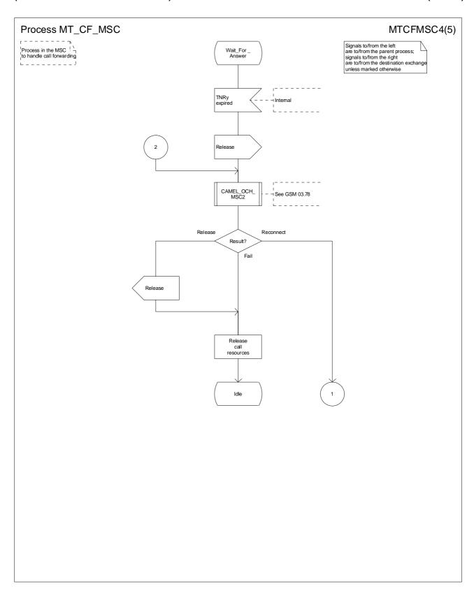
Figure 42d: Process MT\_CF\_MSC (sheet 4)
