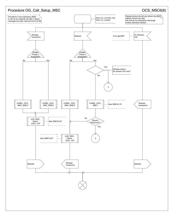
Figure 8f: Procedure Outgoing\_Call\_Setup \_MSC (sheet 6)
