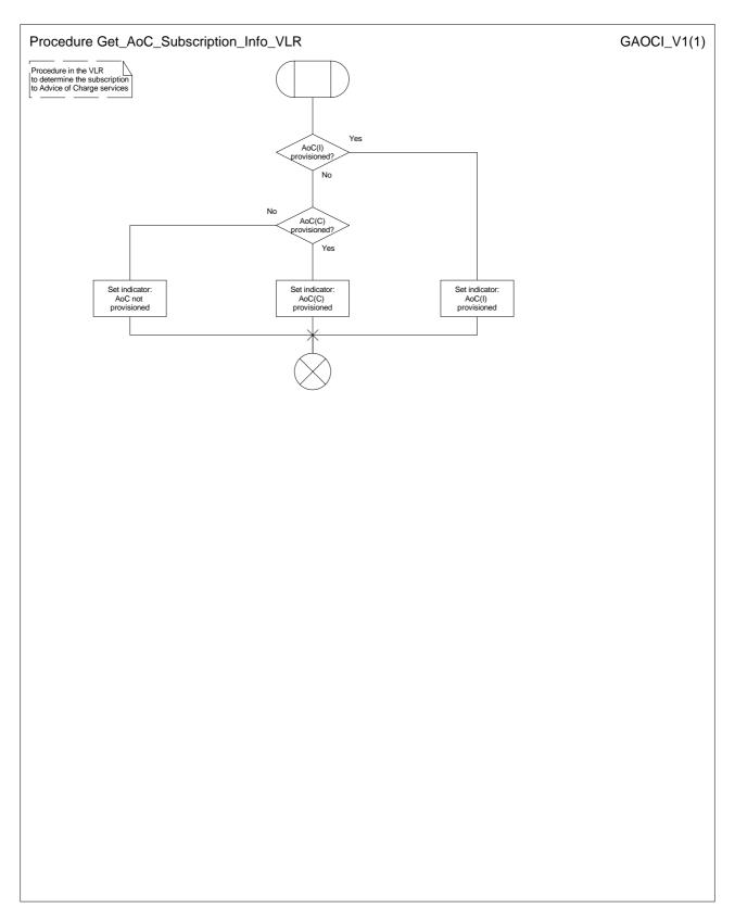
Figure 33: Procedure Get\_AoC\_Subscription\_Info\_VLR
