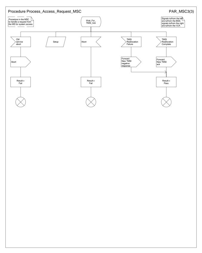
Figure 7c: Procedure Process\_Access\_Request\_MSC (sheet 3)
