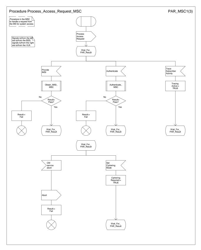
Figure 7a: Procedure Process\_Access\_Request\_MSC (sheet 1)
