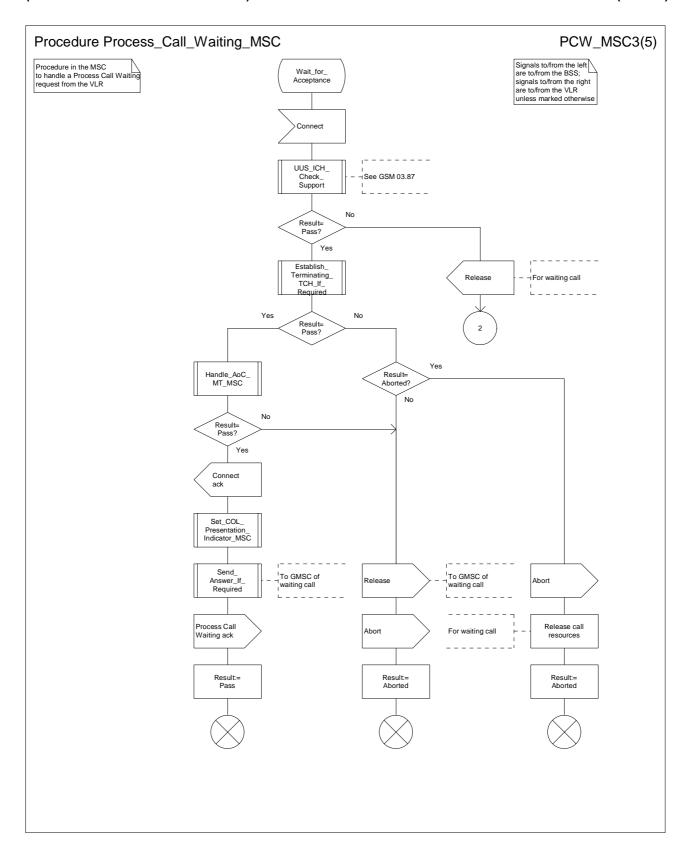
Figure 63c: Procedure Process\_Call\_Waiting\_MSC(sheet 3)
