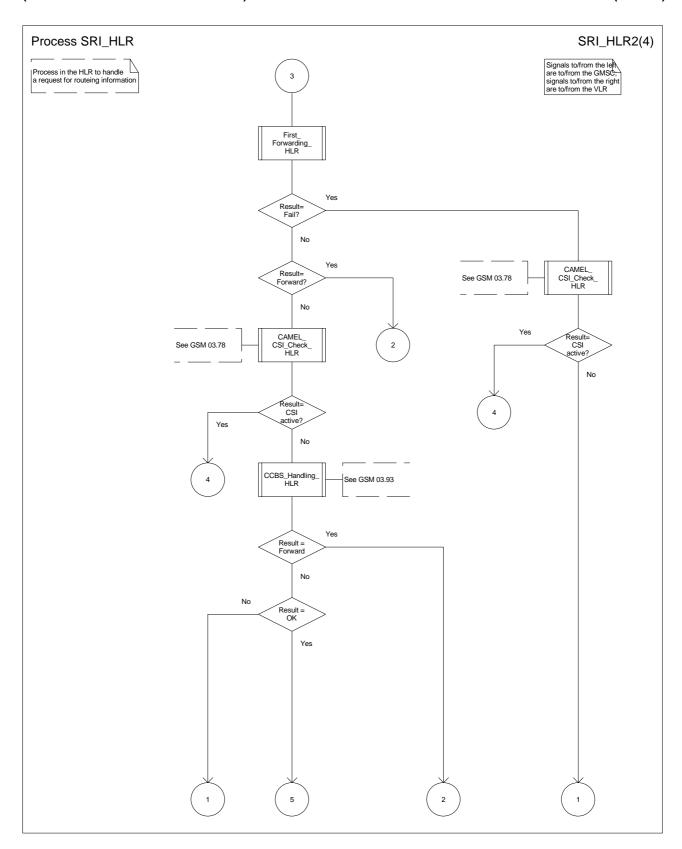
Figure 43b: Process SRI\_HLR (sheet 2)
