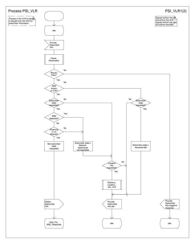
Figure 56a: Process PSI\_VLR (sheet 1)
