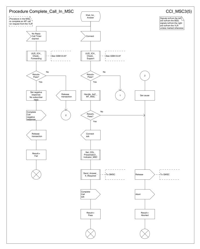
Figure 62c: Procedure Complete\_Call\_In\_MSC (sheet 3)
