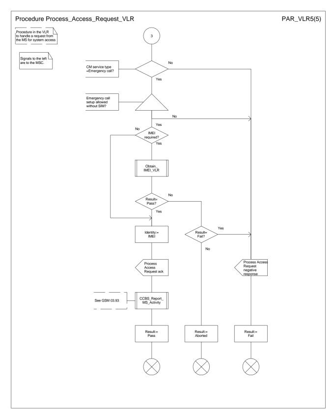
Figure 20e: Procedure Process\_Access\_Request\_VLR (sheet 5)
