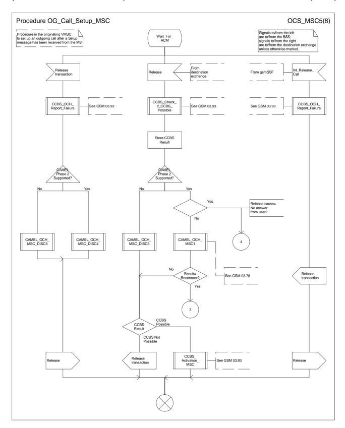
Figure 8e: Procedure Outgoing\_Call\_Setup \_MSC (sheet 5)
