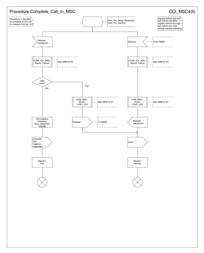
Figure 62d: Procedure Complete\_Call\_In\_MSC (sheet 4)
