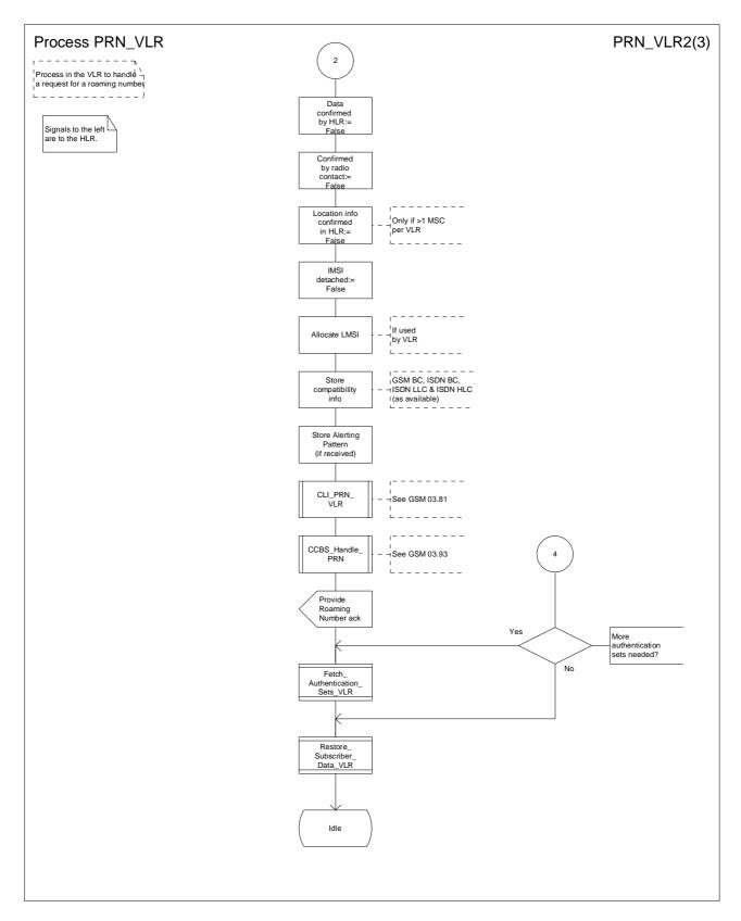
Figure 54b: Process PRN\_VLR (sheet 2)
