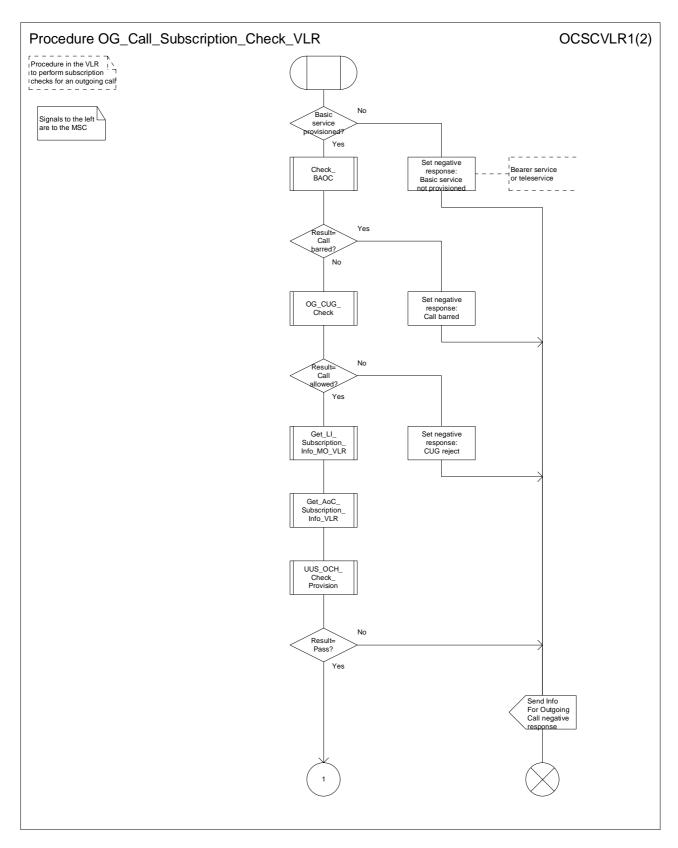
Figure 21a: Procedure OG\_Call\_Subscription\_Check\_VLR (sheet 1)
