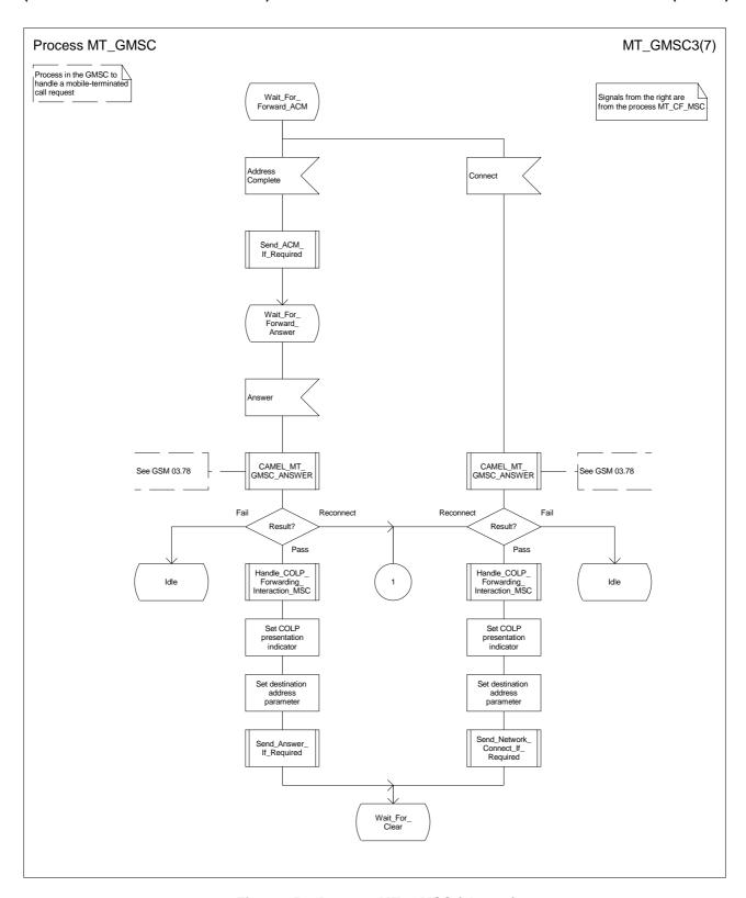
Figure 35c: Process MT\_GMSC (sheet 3)
