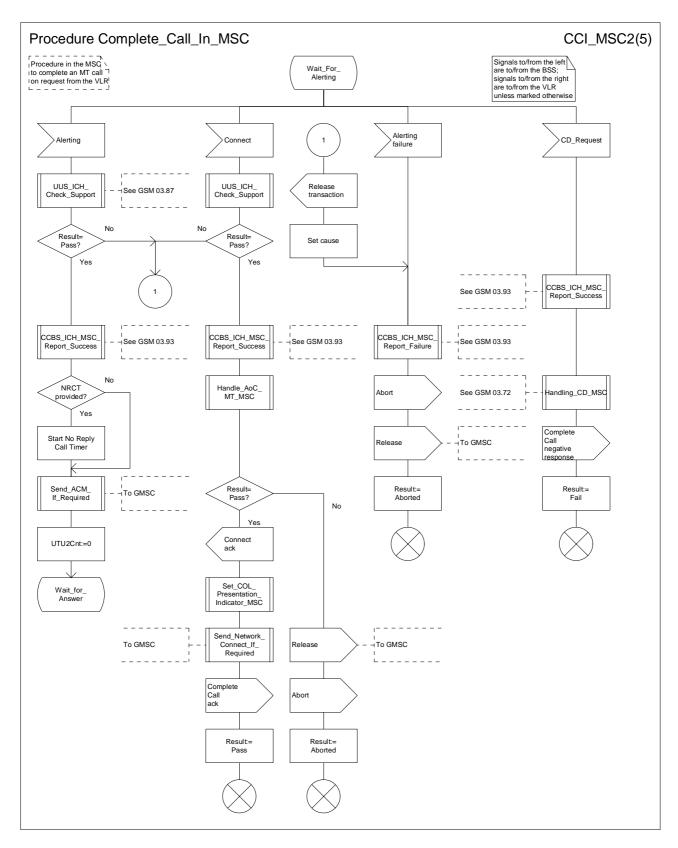
Figure 62b: Procedure Complete\_Call\_In\_MSC (sheet 2)
