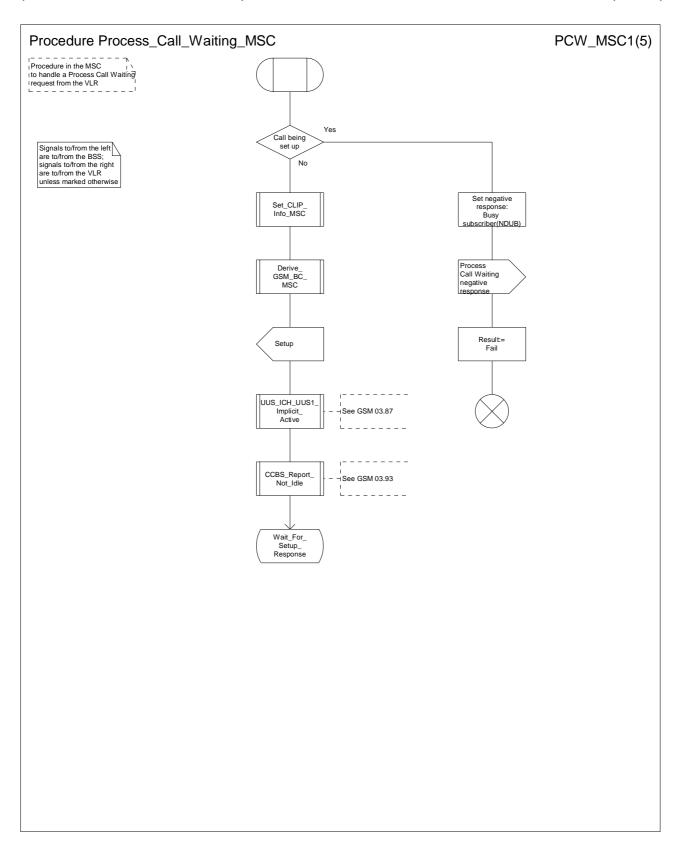
Figure 63a: Procedure Process\_Call\_Waiting\_MSC (sheet 1)
