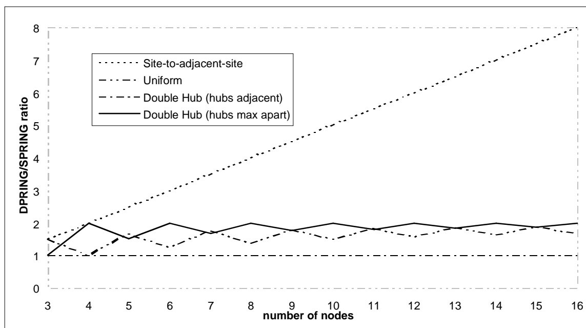
Figure 43: Ratio of required capacity between the MS DPRing and the MS MSPRING for one VC-4 traffic demand
