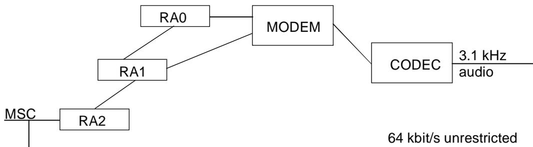
**Figure 8: Protocol structure in the MSC/IWF (transparent)**
