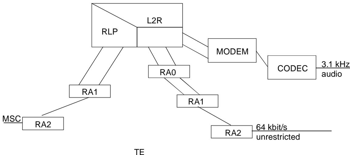
Figure 9: Protocol structure in the MSC/IWF (non-transparent)
