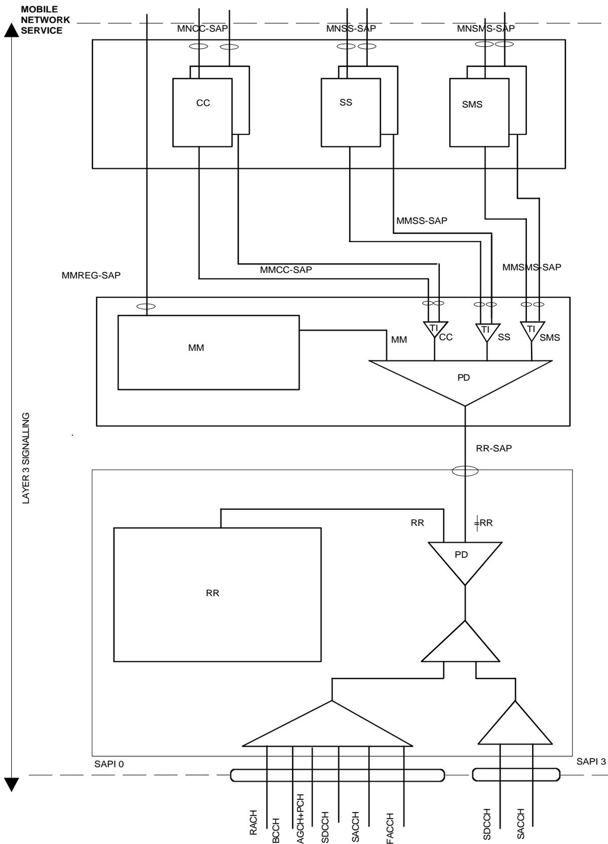
Figure 5.1: Protocol Architecture not supporting GPRS service- MS side
