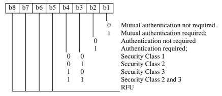
Figure 21: Coding of Security settings
