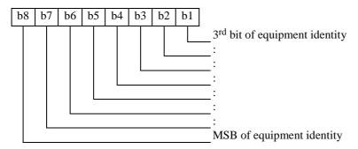
Figure 45: Coding of DMO equipment type and identity
