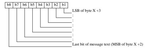
Figure 33: Coding of SDS-1 message text
