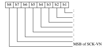
Figure 12: Coding of Static Cipher Key Version Number
