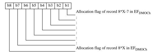
Figure 44: Coding of allocation flags
