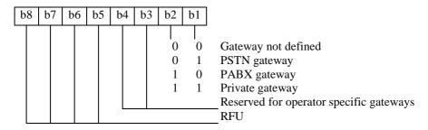
Figure 28: Coding of type of gateway
