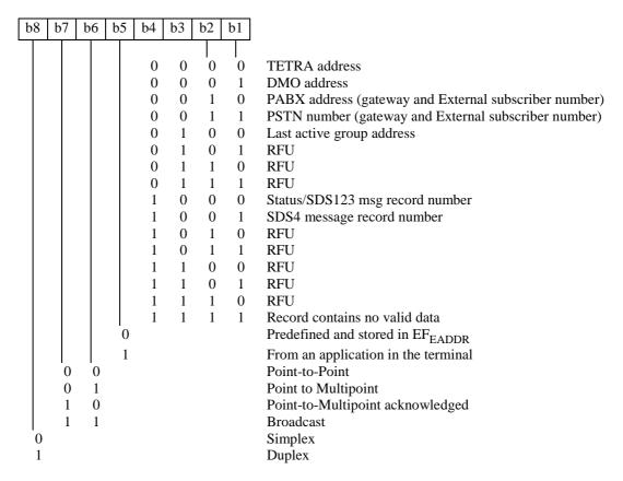
Figure 41: Coding of Emergency call definition
