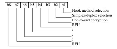
Figure 29: Coding of call modifier bytes 1 and 2
