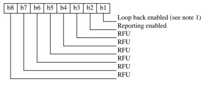
NOTE 1: Loop back enabled and security/authentication disabled (see ETS 300 394-2 [10]). NOTE 2: The coding '00' means normal operation.
