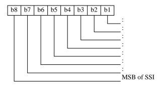
Figure 27: Coding of gateway SSI
