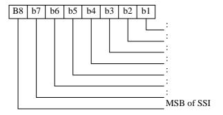
Figure 38: Coding of SSI
