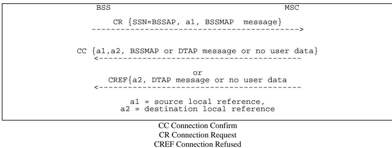
**Figure 1/08.06: Set-up of SCCP connections on the first BSS/MSC interface**
