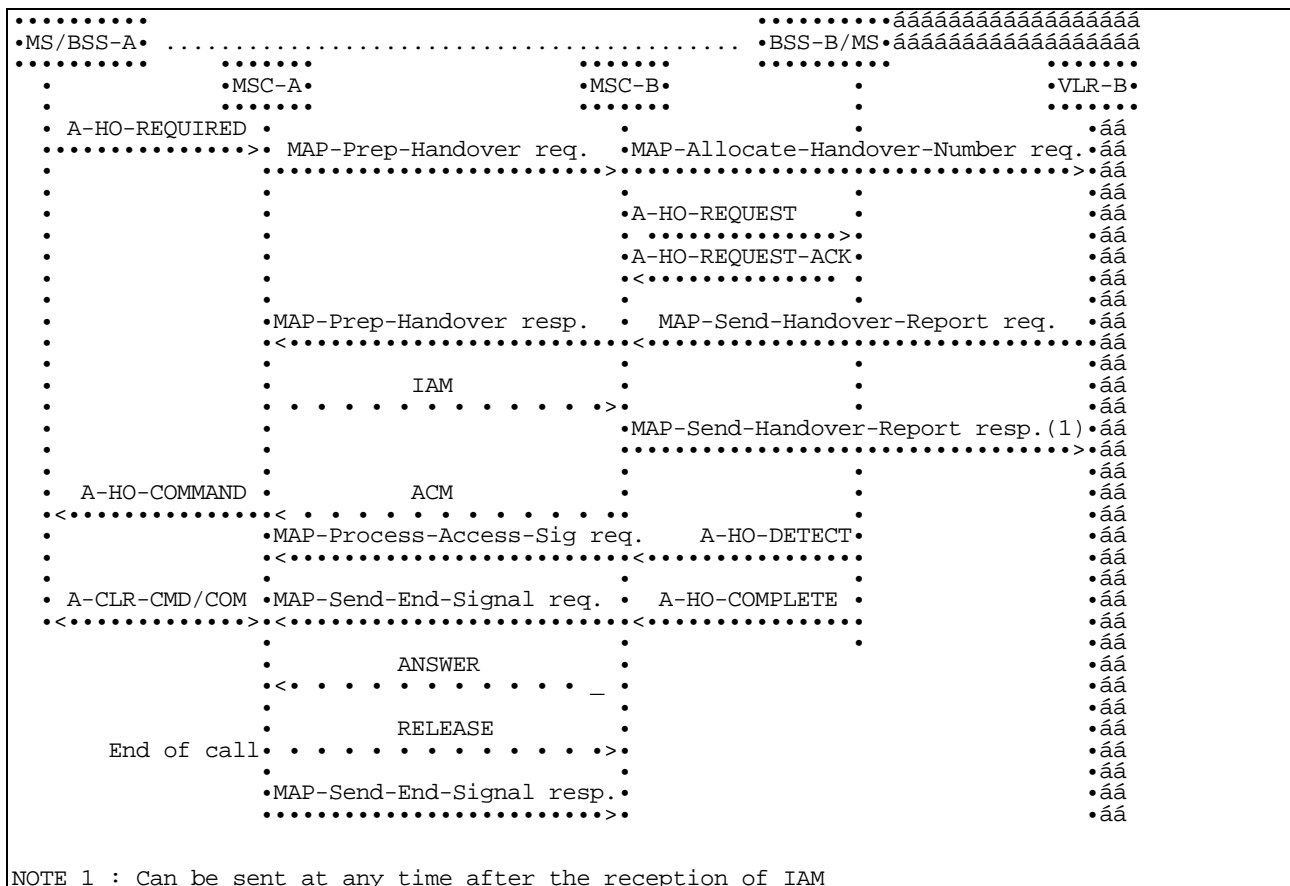
Figure 5: Basic Handover Procedure requiring a circuit connection
