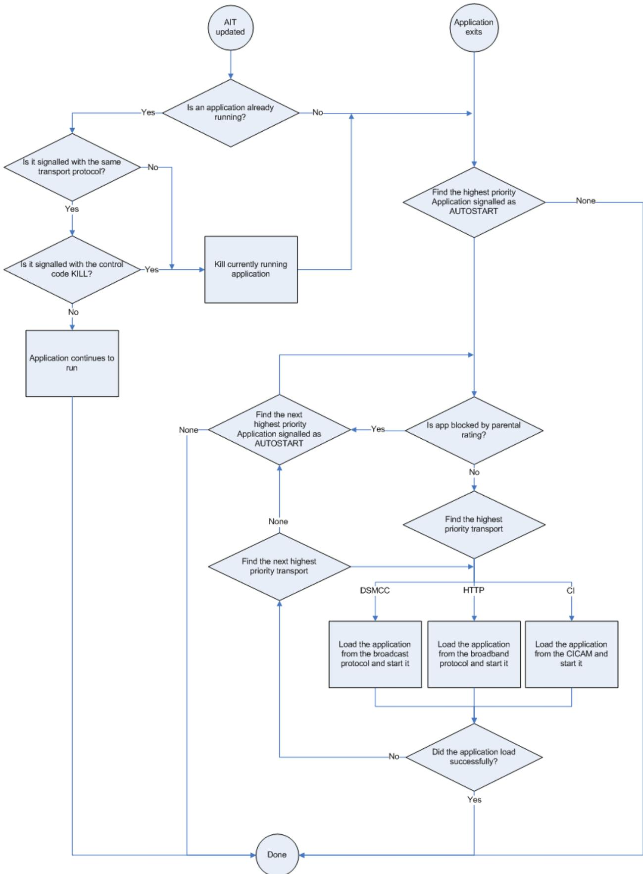
Figure 14: Behaviour while a broadcast service is selected
