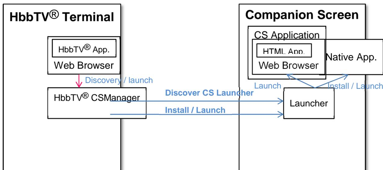
**Figure 31: Architecture for launching a CS application**
