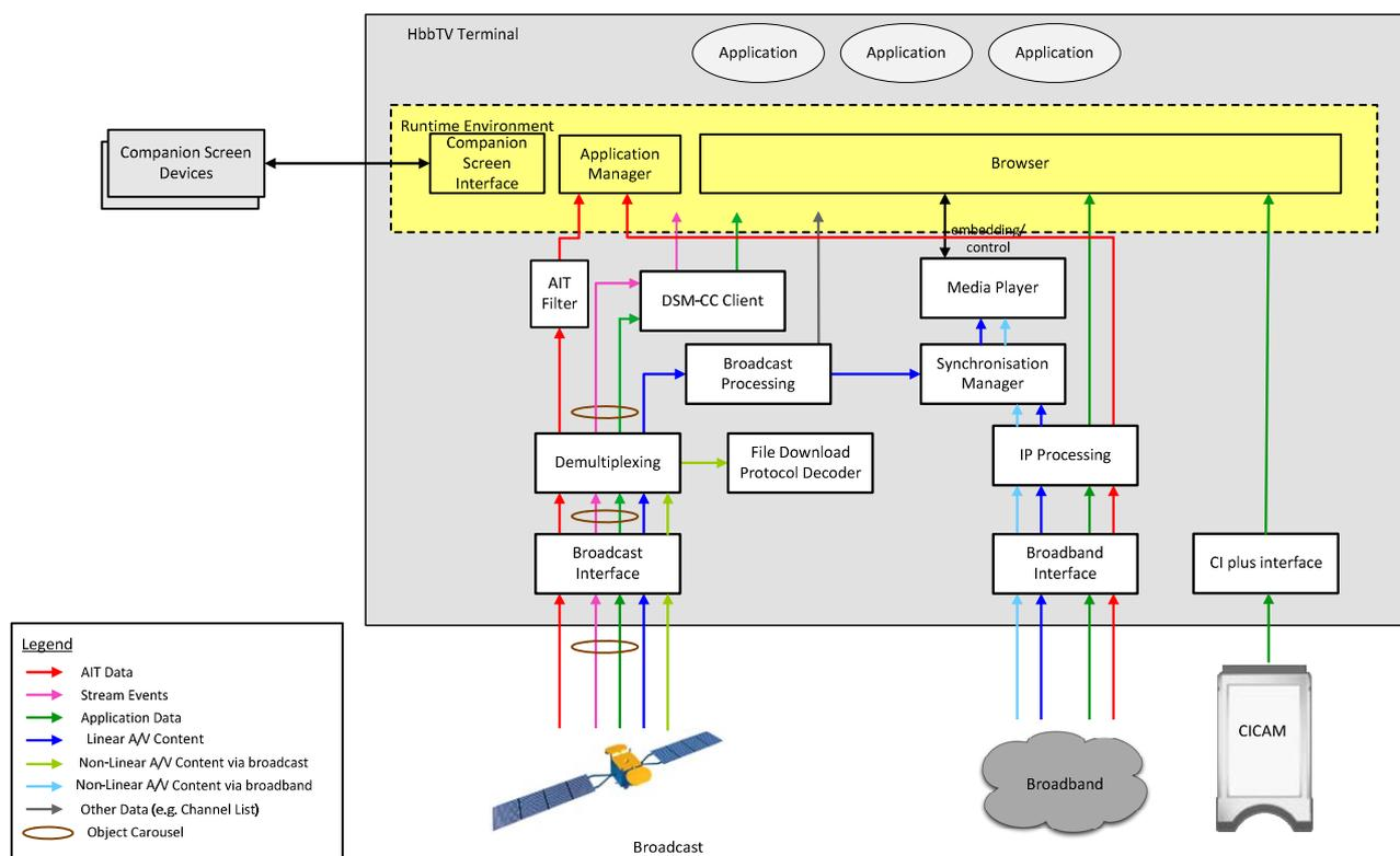
**Figure 2: Functional components of a hybrid terminal**
