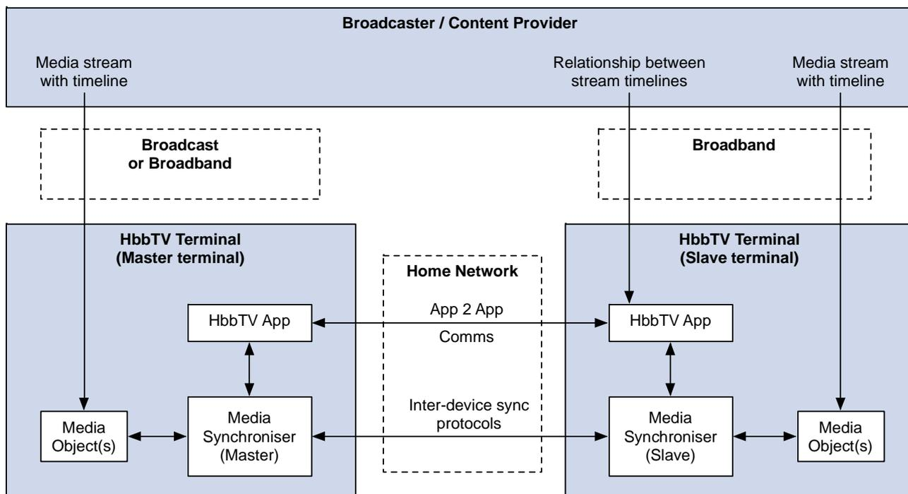
**Figure 20: Relationship between MediaSynchroniser object and HbbTV<sup>®</sup> application for inter-device synchronization with a slave terminal**
