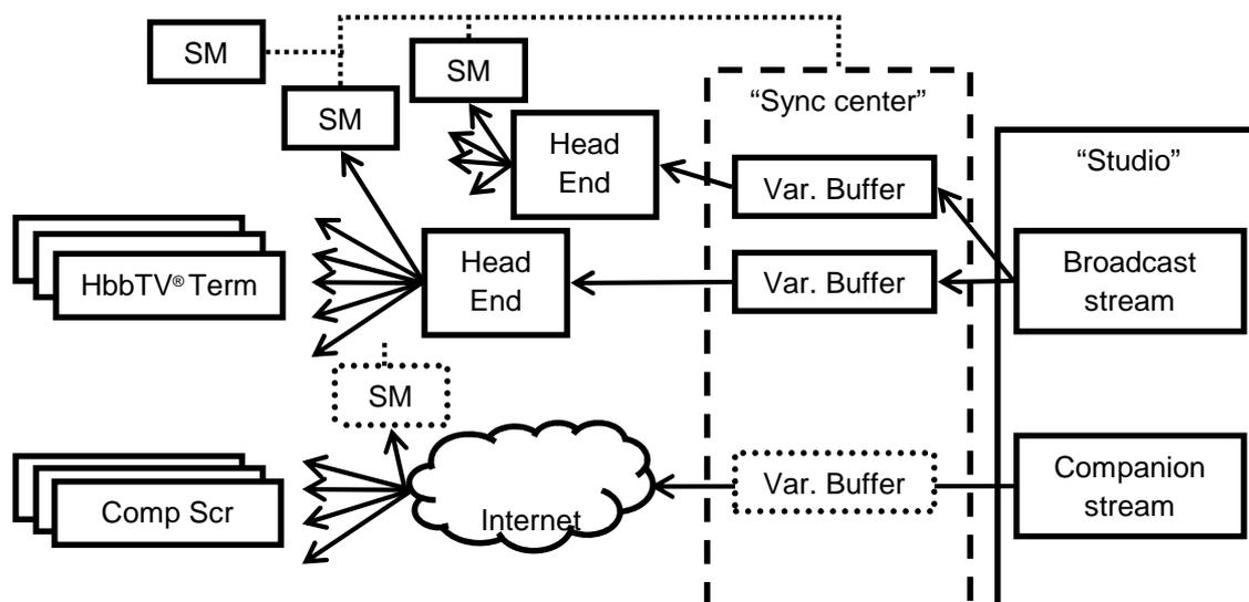
Figure G.1: Architecture for delay management and equalisation
