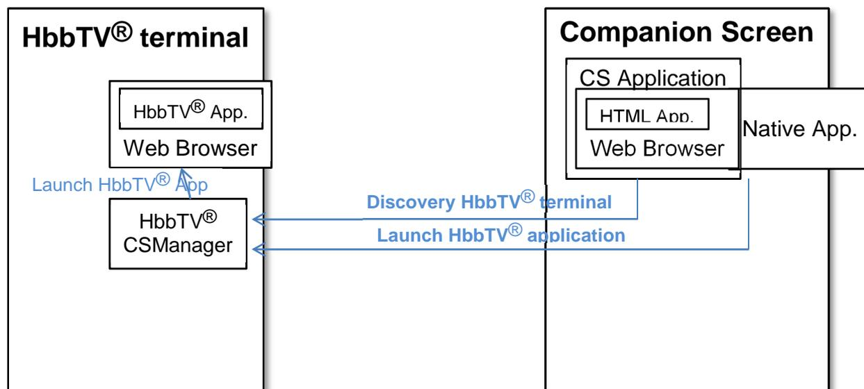
**Figure 33: Architecture for remotely launching HbbTV<sup>®</sup> applications**
