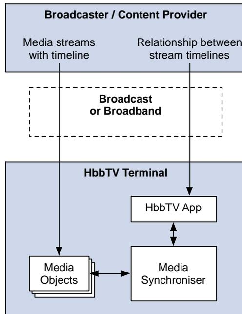
**Figure 17: Relationship between MediaSynchroniser object and HbbTV<sup>®</sup> application for multi-stream synchronization**
