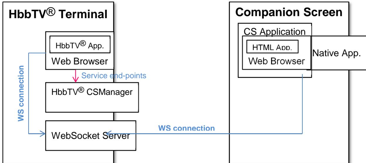
**Figure 32: Architecture for application to application communication**
