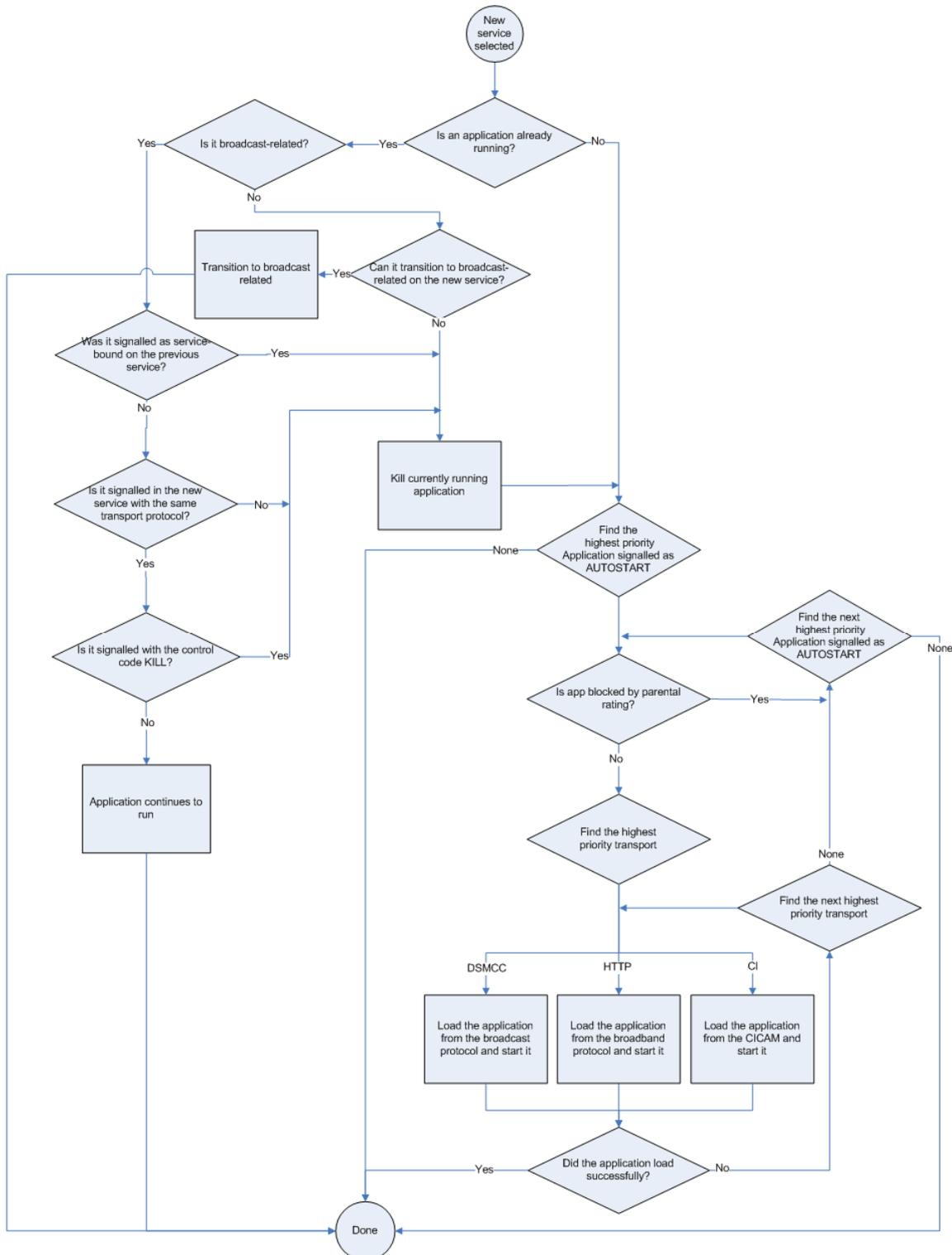
Figure 13: Behaviour when selecting a broadcast service
