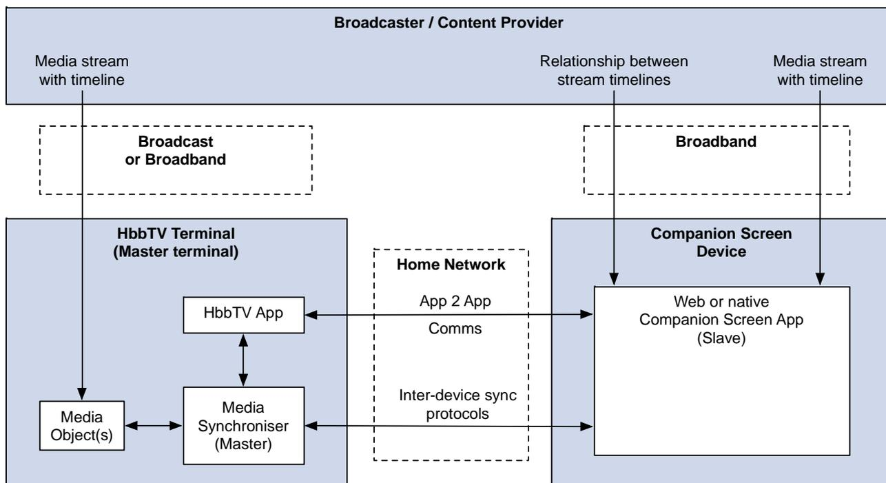
**Figure 19: Relationship between MediaSynchroniser object and HbbTV<sup>®</sup> application for inter-device synchronization with a CSA**
