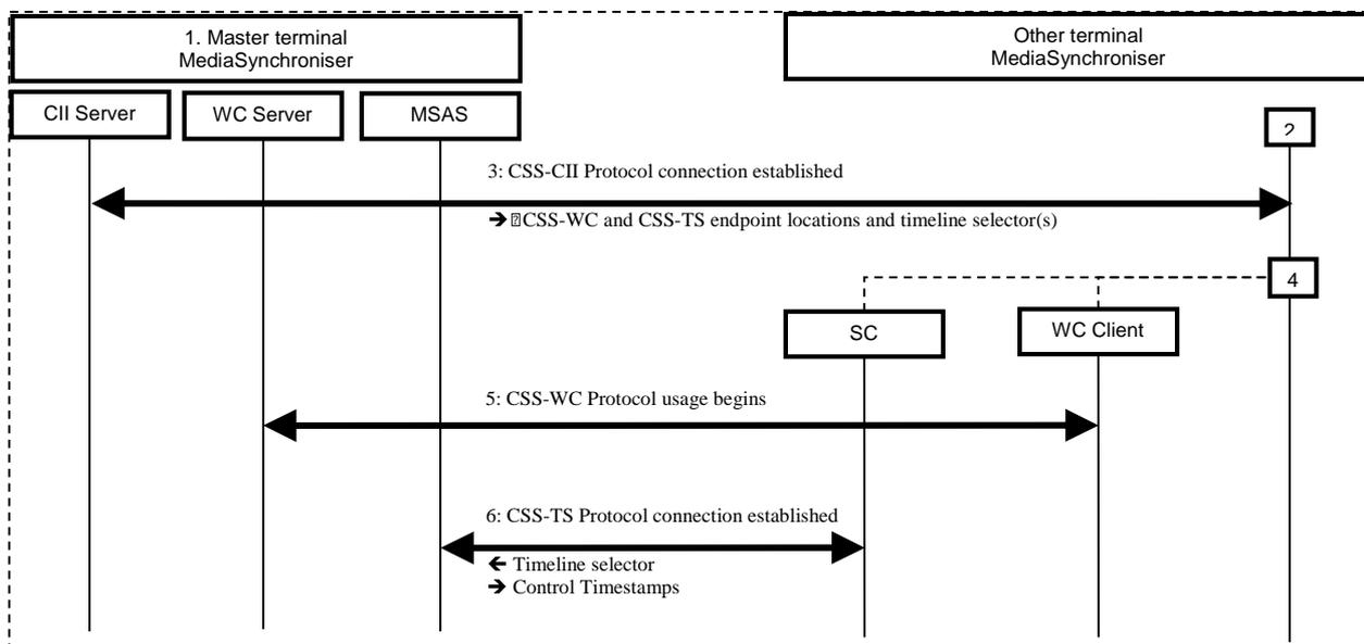
**Figure 25: Protocol interactions for inter-device timeline synchronization**
