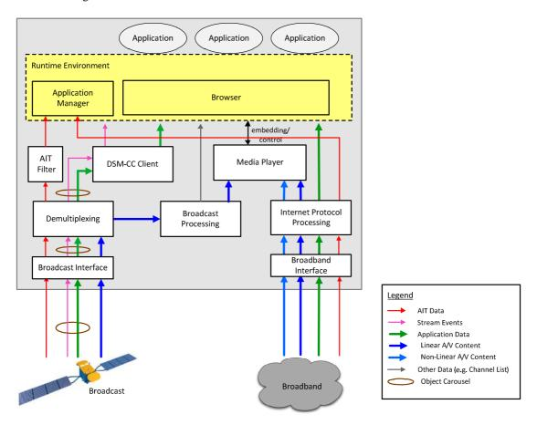
Figure 2: Functional components of a hybrid terminal
