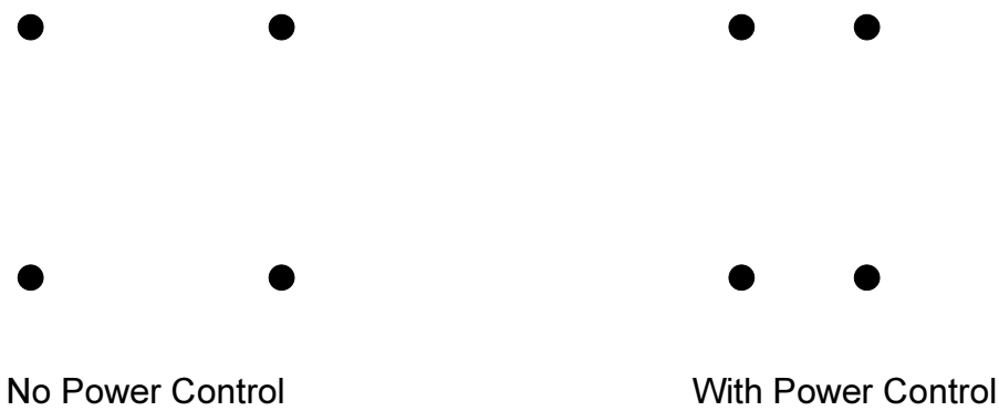
Figure 9-5: Downlink power control on HOM – QPSK
