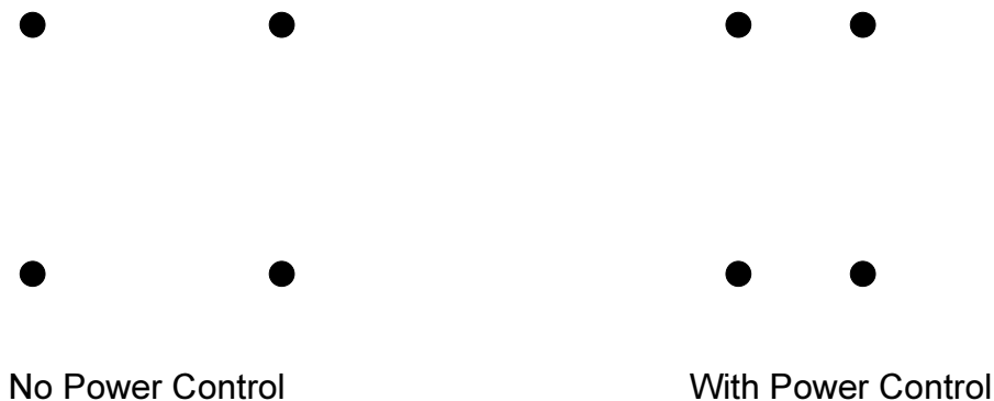
Figure 9-5: Downlink power control on HOM – QPSK
